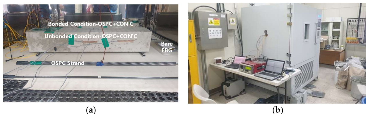
Figure 12. View of temperature-compensation experiments (a) Installation of specimen, (b) View of measurement.
