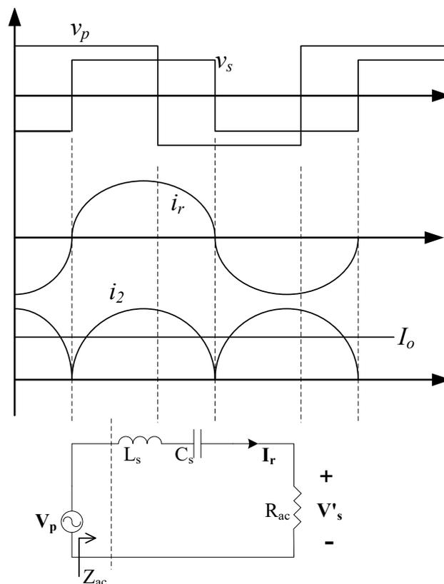
Figure 5. The typical steady-state waveforms of Method II.
