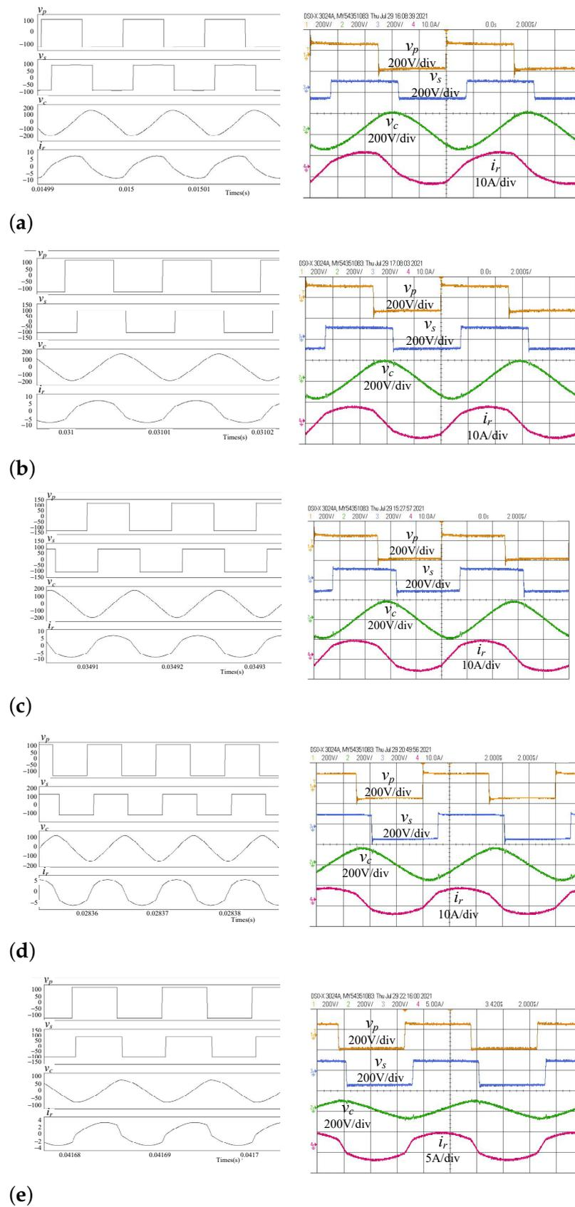
**Figure 8.** Simulated (left) and experimental (right) waveforms of  $v_p, v_s, v_c, i_r$  with Method I: (a)  $V_o = 84$  V, CC; (b)  $V_o = 108$  V, CC; (c)  $V_o = 120$  V,  $I_o = 5$  A; (d)  $I_o = 4$  A, CV; (e)  $I_o = 2.5$  A, CV.
