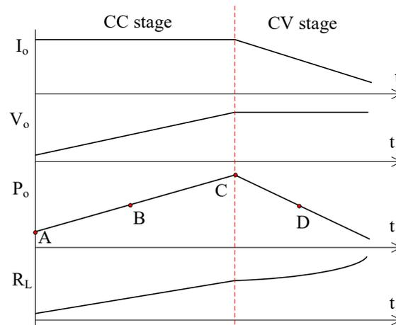
**Figure 1.** Variations of voltage, current, and power in a typical charging process.
