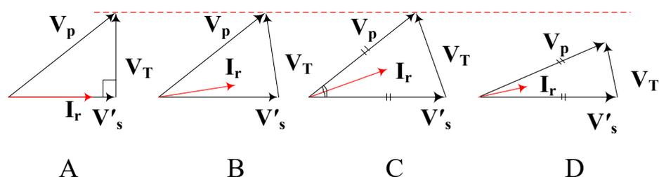
Figure 4. Phasor diagram of the converter of Method I.
