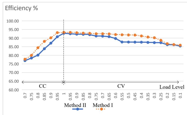
**Figure 11.** Measured efficiency of two proposed modulation methods.
