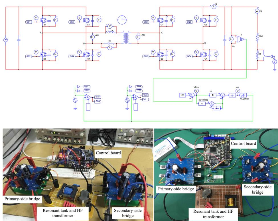
Figure 7. Simulation block diagram and experimental prototype
