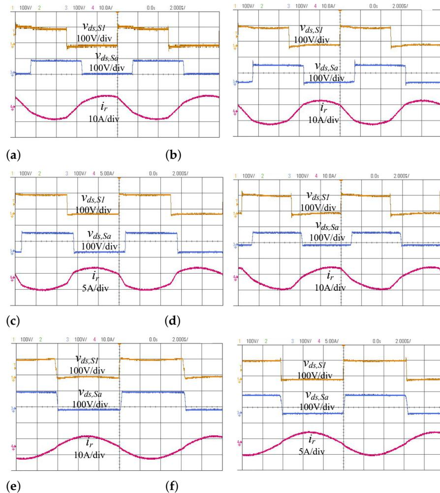
**Figure 10.** Switch voltages of  $S_1$ ,  $S_a$  and resonant current  $i_r$ : (a)  $V_o = 84$  V, CC, Method I; (b)  $V_o = 120$  V,  $I_o = 5$  A, Method I; (c)  $I_o = 2.5$  A, CV, Method I; (d)  $V_o = 84$  V, CC, Method II; (e)  $V_o = 120$  V,  $I_o = 5$  A, Method II; (f)  $I_o = 2.5$  A, CV, Method II.
