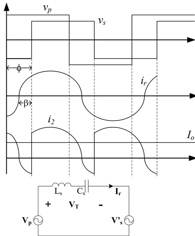
Figure 3. The typical steady-state waveforms of Method I.
