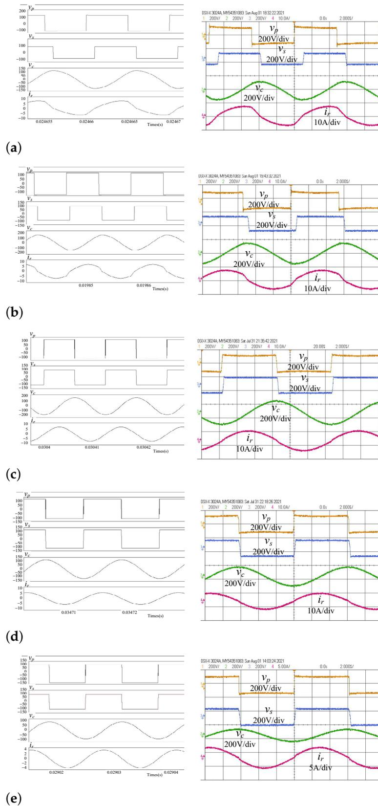
**Figure 9.** Simulated (left) and experimental (right) waveforms of  $v_p, v_s, v_c, i_r$  with Method II: (a)  $V_o = 84\text{ V, CC}$ ; (b)  $V_o = 108\text{ V, CC}$ ; (c)  $V_o = 120\text{ V, } I_o = 5\text{ A}$ ; (d)  $I_o = 4\text{ A, CV}$ ; (e)  $I_o = 2.5\text{ A, CV}$ .
