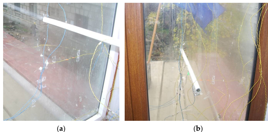
Figure 14. Condensation phenomena inside the DSF channel (a) exterior glazing—view from inside the channel, (b) interior glazing—view from inside the interior room.
