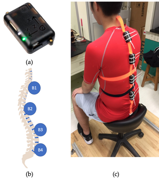
Figure 2. (a) Nine-axis inertial measurement units (NGIMU); (b) distribution of IMUs where blue dots represent positions of IMUs relative to subjects' spines: B1 was positioned at T1, B4 was positioned at L5, and B2 and B3 were evenly distributed between S1 and S4; and (c) prototype of the sitting posture recognition device.
