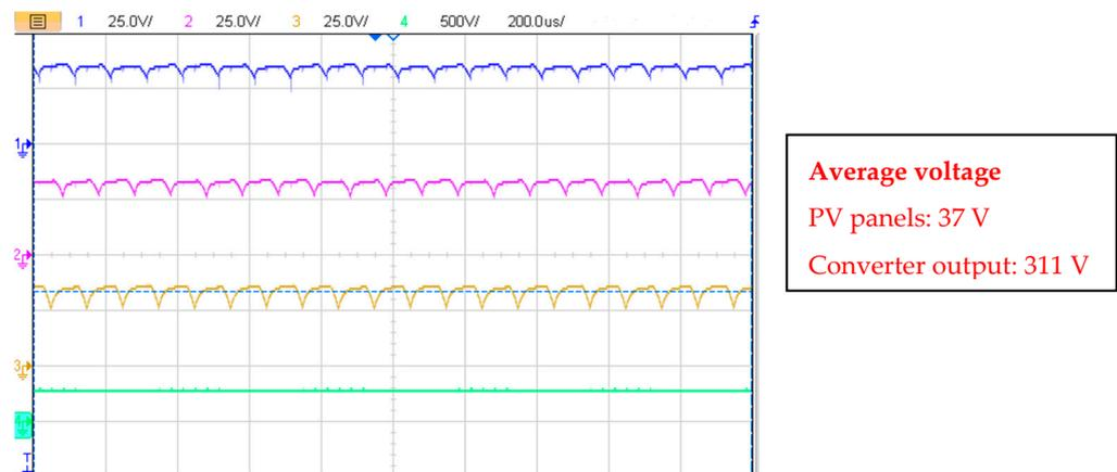
**Figure 18.** Experimental waveforms. Input voltages: PV panel 1 (blue), PV panel 2 (pink), and PV panel 3 (yellow); scale: 25 V/div. Converter output voltage (green); scale: 500 V/div. Base time: 200 μs/div.
