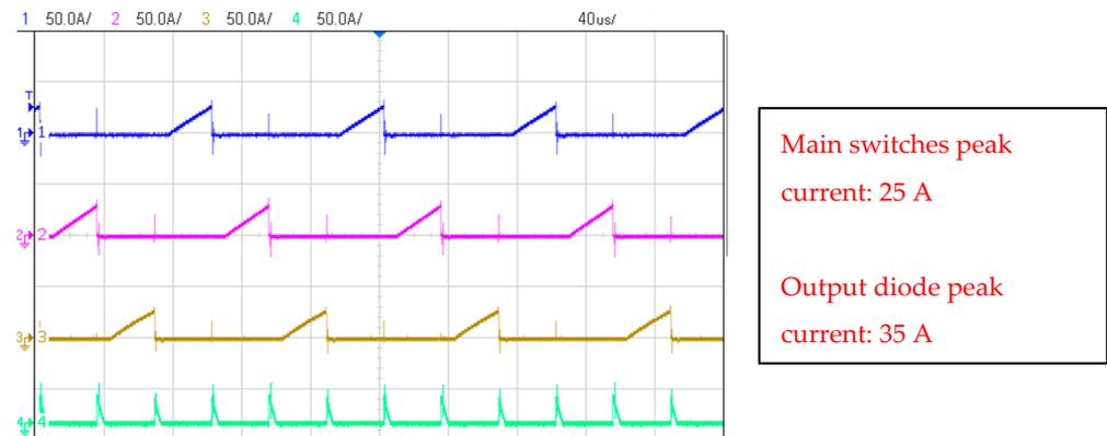
**Figure 22.** Experimental waveforms near sunset. Current: main switch 1 (yellow), main switch 2 (pink), and main switch 3 (yellow); scale 50 A/div. Output diode current (green); scale: 50 A/div. Base time Base time 40  $\mu$ s/div.
