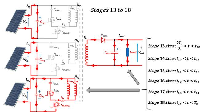
Figure 9. Schematic of stages 13 to 18, time:  $2T_s/3 < t < T_s$ .
