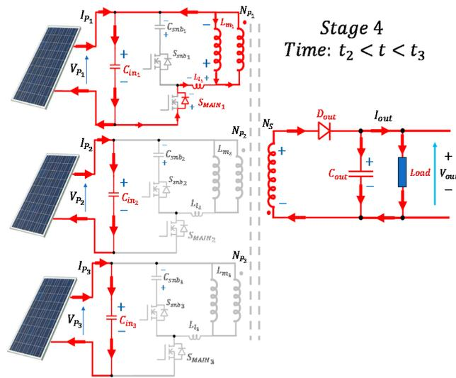
Figure 5. Stage 4, time:  $t_2 < t < t_3$ .
