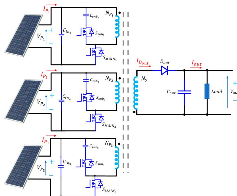
Figure 1. Topology proposed, with  $N = 3$  PV panels.
