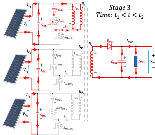
Figure 4. Stage 3, time:  $t_1 < t < t_2$ .
