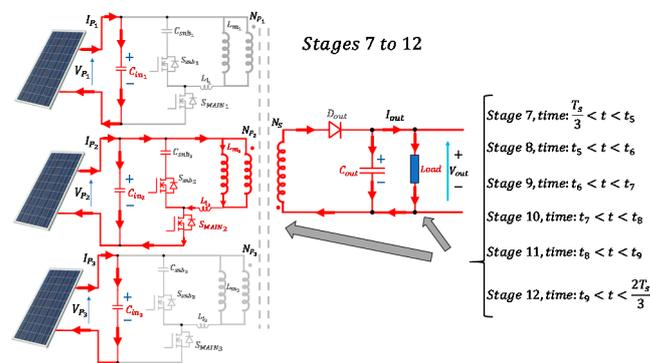
Figure 8. Schematic of stages 7 to 12, time:  $T_s/3 < t < 2T_s/3$ .
