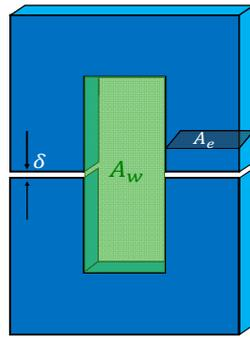
Figure 12. O-type ferrite core for each flyback transformer.
