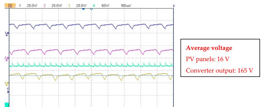
**Figure 23.** Experimental waveforms near sunset: Input voltages: PV panel 1 (blue), PV panel 2 (pink), and PV panel 3 (yellow); scale: 25 V/div. Converter output voltage (green); scale: 50 V/div. Base time 100  $\mu$ s/div.
