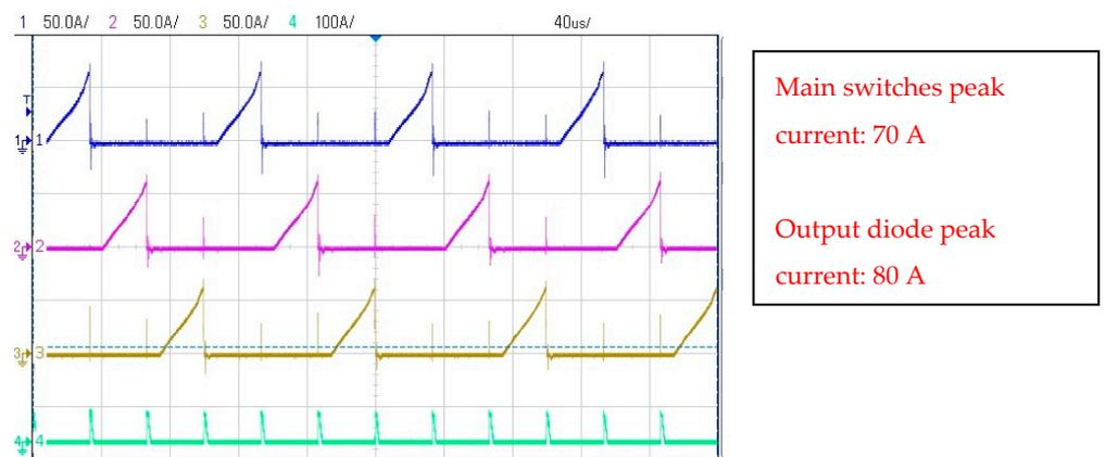
**Figure 21.** Experimental waveforms. Current: main switch 1 (yellow), main switch 2 (pink), and main switch 3 (yellow); scale 50 A/div. Output diode current (green); scale: 100 A/div. Base time 40  $\mu$ s/div.
