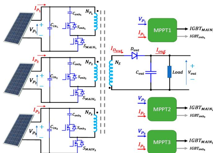
Figure 10. Schematic of the MPPT for the topology proposed.
