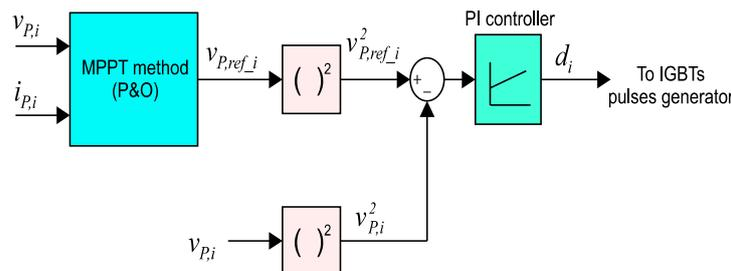
Figure 11. MPPT control scheme for each PV module.
