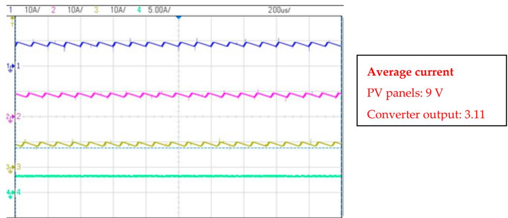
**Figure 19.** Experimental waveforms. PV panels’ currents: PV panel 1 (blue), PV panel 2 (pink), and PV panel 3 (yellow); scale: 10 A/div. Converter’s output current (green); scale: 5 A/div. Base time: 200  $\mu$ s/div.
