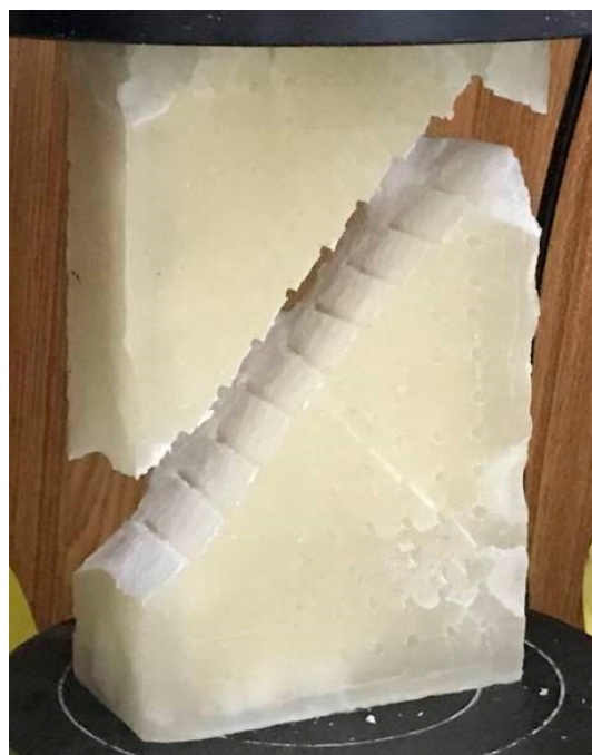
Figure 3. Fracture process of mixed paraffin model ice.
