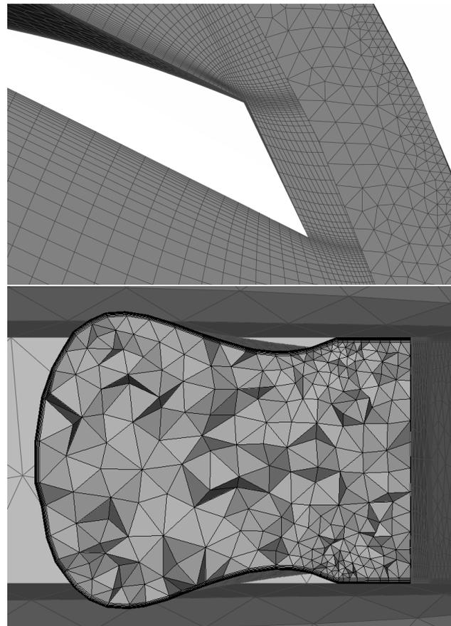
Figure 10. Detail of the impeller (top) and volute (bottom) mesh for the baseline design, medium mesh.
