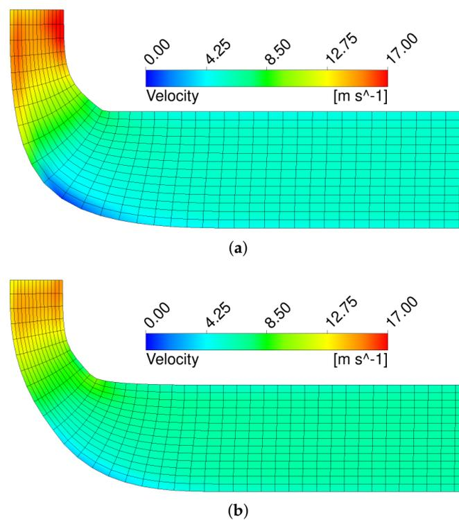
**Figure 19.** Velocity field in the meridional channel for the baseline (a) and the optimized (b) geometries.
