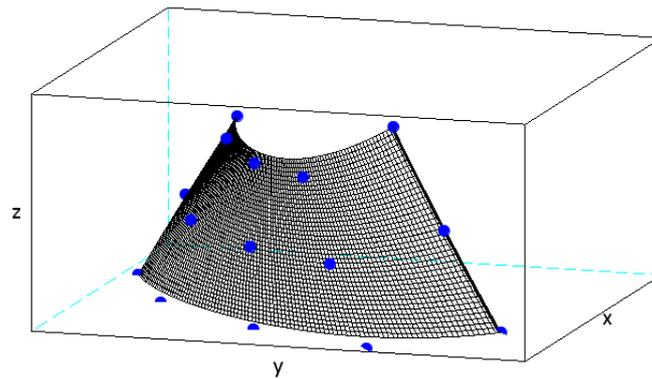
Figure 5. Control points and camber surface for the blade.
