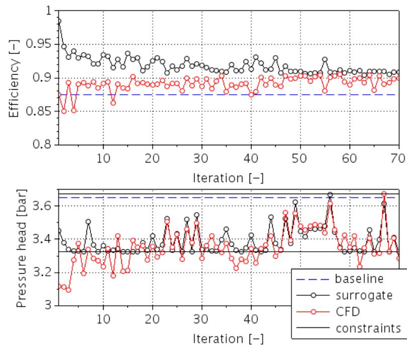
**Figure 12.** Evaluation of the design from the SOGA with the surrogate and CFD simulation: efficiency (**top**) and total pressure head (**bottom**).
