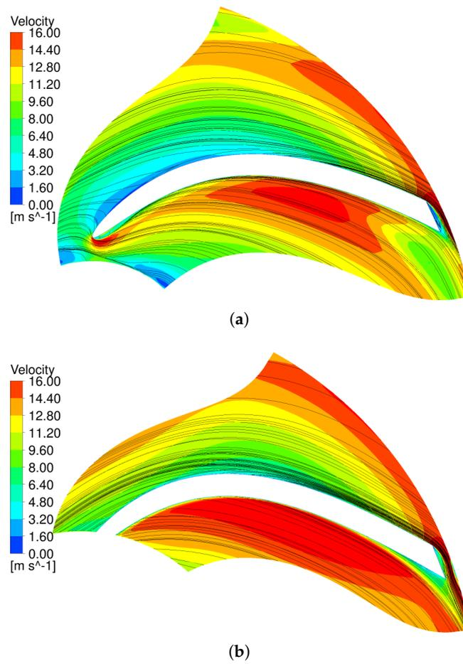
**Figure 18.** Velocity contours and streamline in the plane  $z = 5$  mm for the baseline (a) and the optimized (b) geometries.
