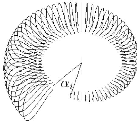
Figure 8. Baffle tongue angle controlled by the design variable  $\alpha_i$ .
