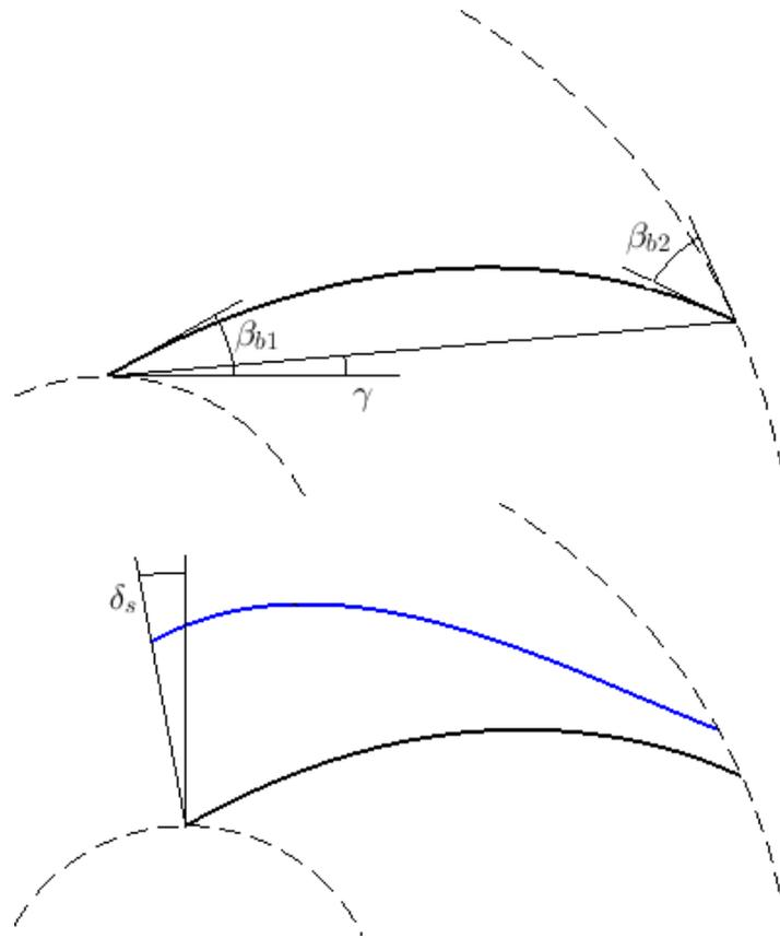
**Figure 2.** Main symbols for the impeller geometry (**top**), and impeller blade (**middle, bottom**).
