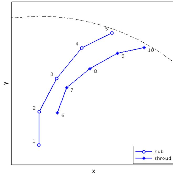
Figure 3. Control points for the camber surface at the hub and shroud.
