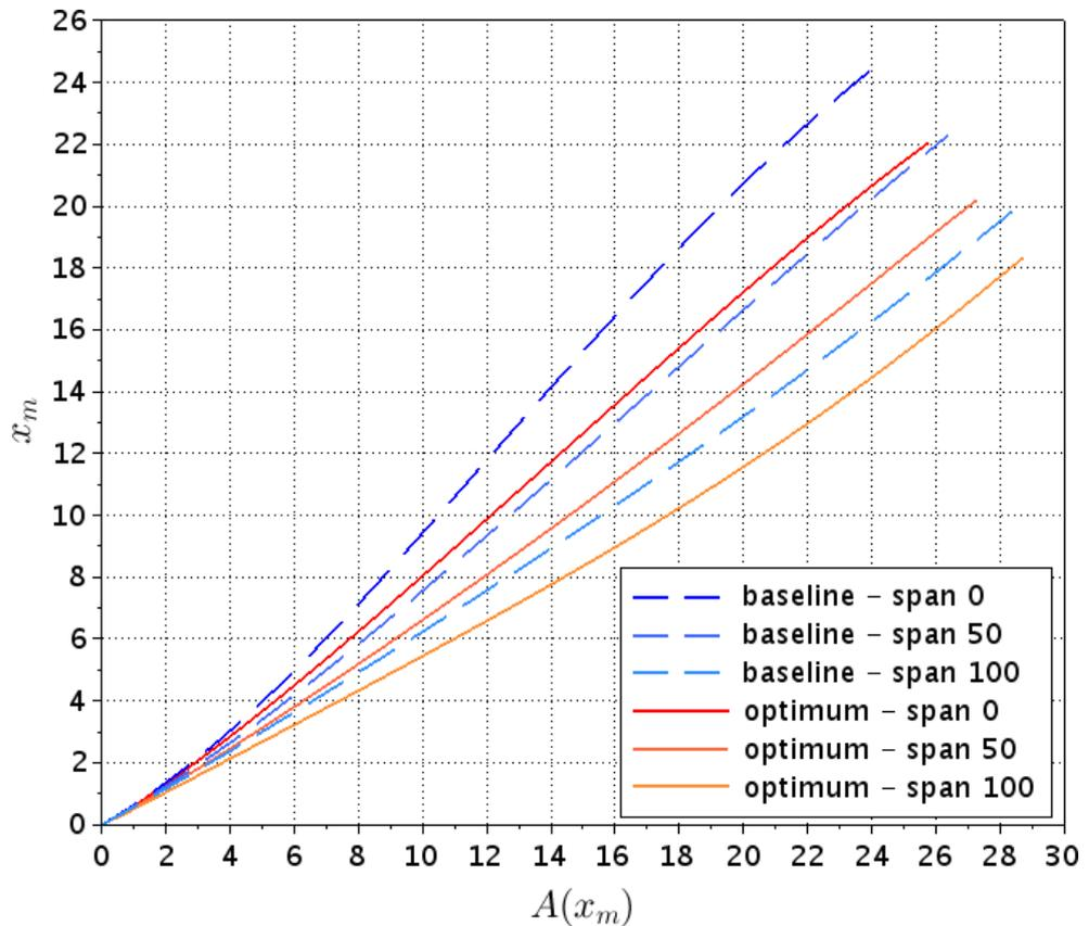
Figure 14. Profiles of the blade camberline in the conformal mapping plane for the baseline and optimized geometry.
