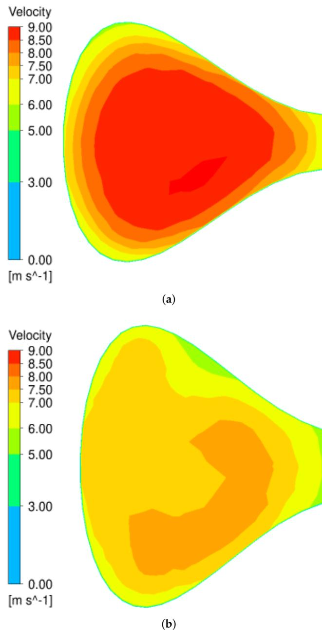
**Figure 22.** Velocity field at the volute outlet for the baseline (a) and the optimized (b) geometries.
