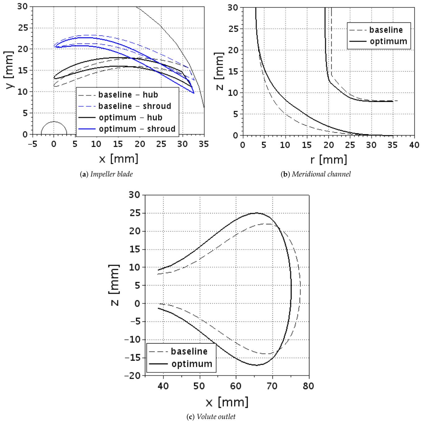
Figure 15. Comparison between baseline and optimized geometries.
