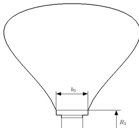
Figure 7. Vaneless diffuser width,  $b_3$  and outlet radius,  $R_3$ .
