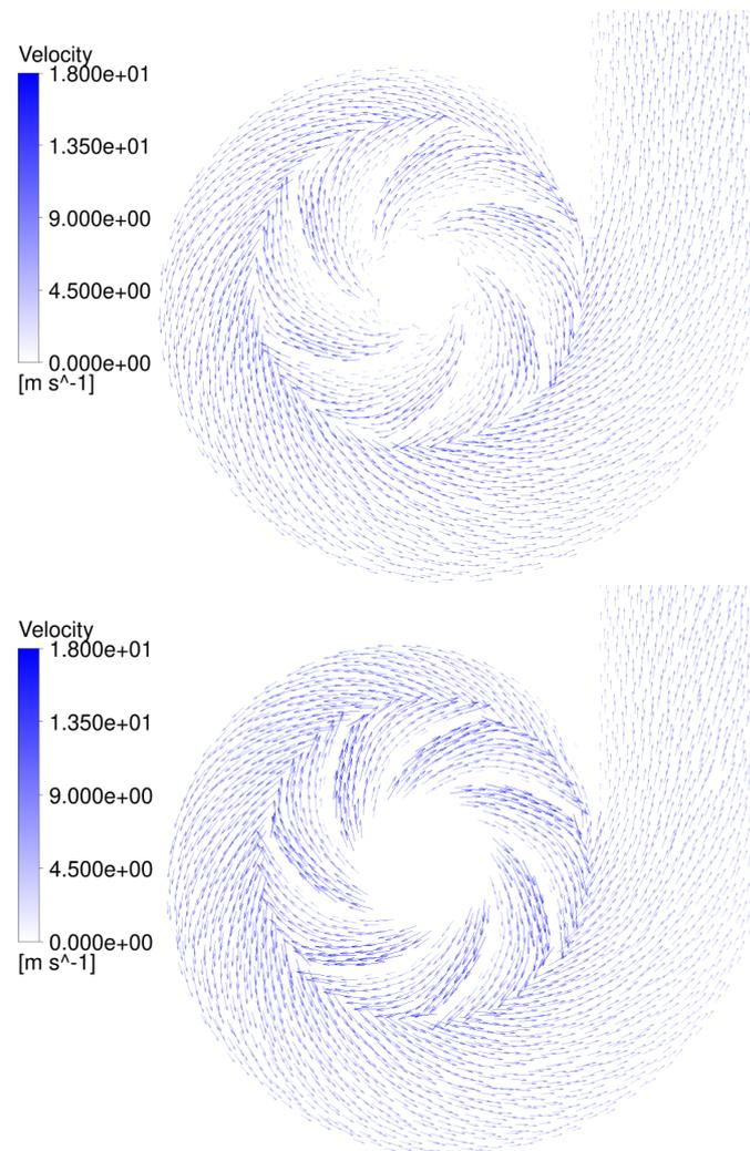
**Figure 23.** Velocity vectors (relative velocity for the impeller and absolute velocity for the volute) for the baseline (**top**) and the optimized (**bottom**) geometries,  $z = 5$  mm.
