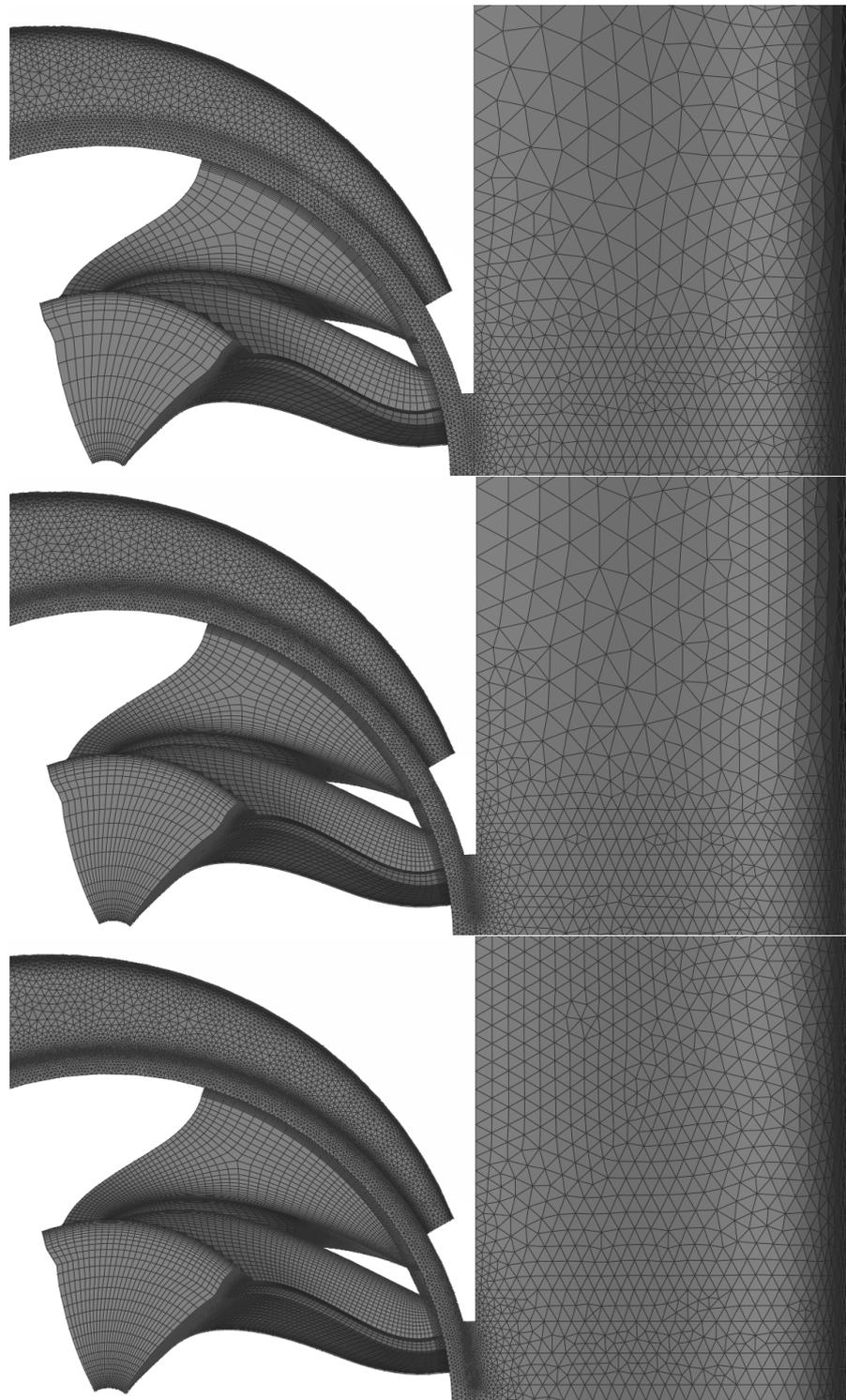
**Figure 9.** Detail of the coarse (**top**), medium (**middle**) and fine (**bottom**) mesh for the baseline design.
