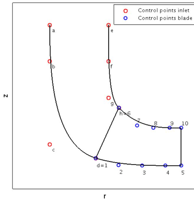
Figure 4. Control points for the meridional channel.
