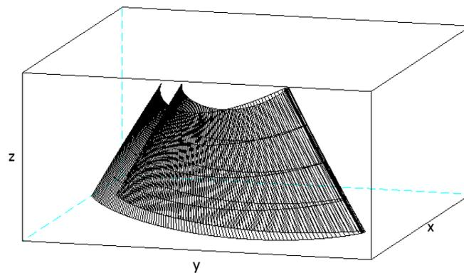
Figure 6. Pressure side and suction side of the blade after applying the thickness function.
