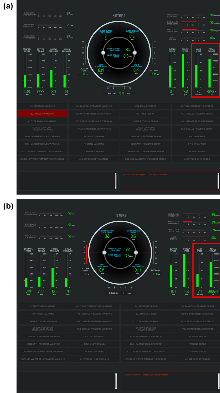
Figure 12. Simulation test results induced by: (a) thrust increase; and (b) shield jack speed decrease (refer to values in red boxes).
