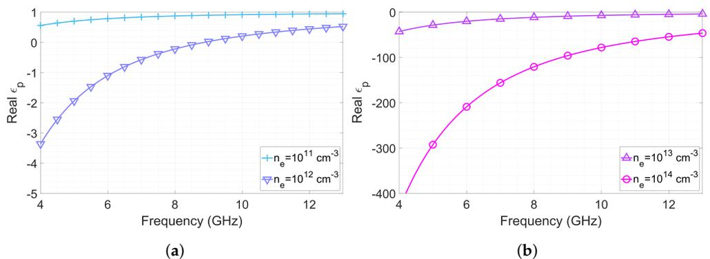
**Figure 9.** Plasma tube real permittivity at  $\nu_p = 10^{10} \text{ 1/s}$  as a function of the frequency for different electron densities  $n_e$  (a)  $n_e = 10^{11}$  and  $n_e = 10^{12} \text{ cm}^{-3}$ ; (b)  $n_e = 10^{13}$  and  $n_e = 10^{14} \text{ cm}^{-3}$ .
