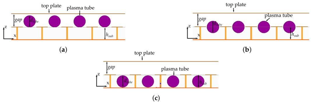
**Figure 8.** Different configurations of the relative position of the tubes with respect to the substrate and the mushroom cap. (a) top of the substrate and mushroom metallic cap; (b) half inserted in the substrate, in-line with the mushroom metallic cap; (c) below the mushroom metallic cap.
