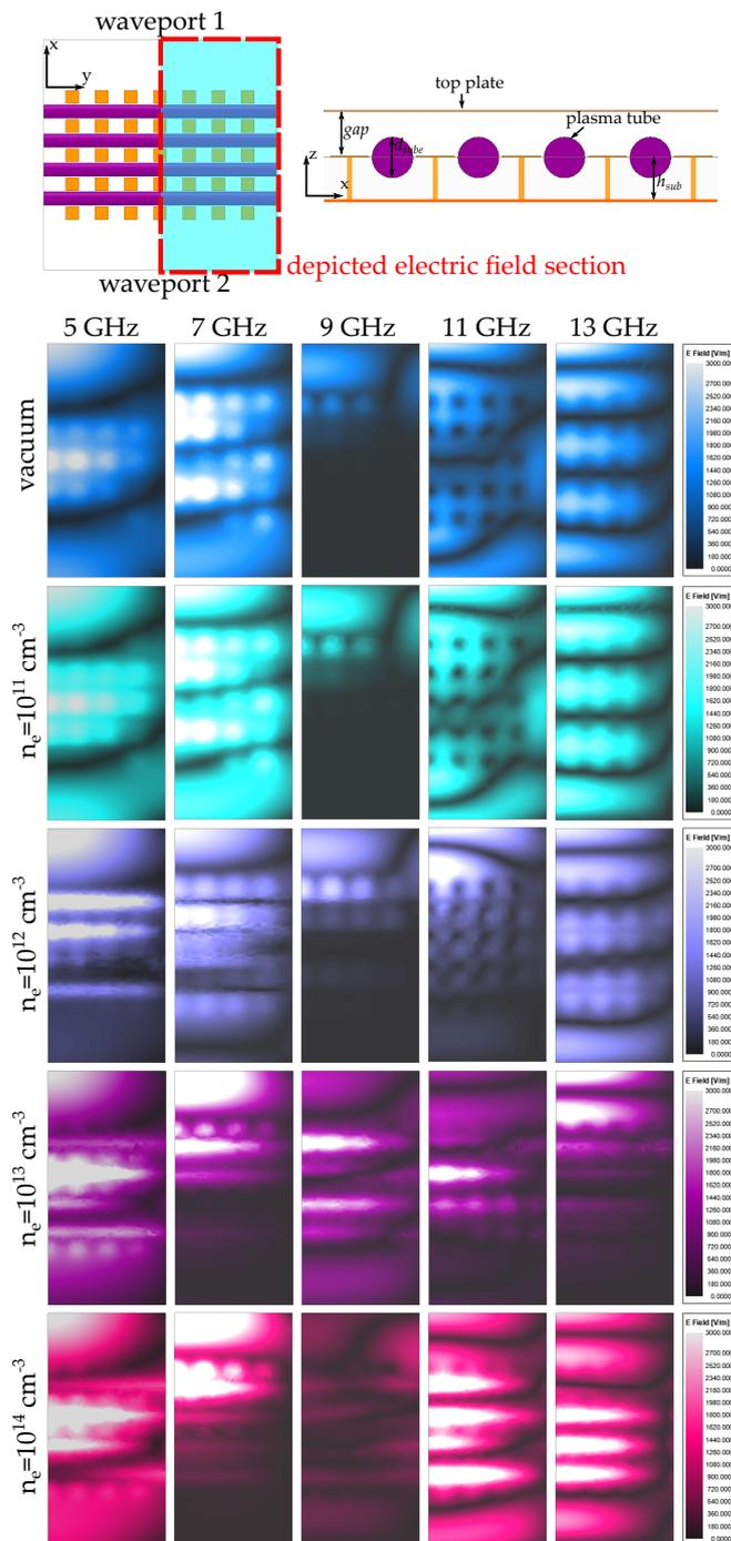
**Figure 11.** Simulated electric field magnitude at five different frequencies over the assessed band (5 GHz, 7 GHz, 9 GHz, 11 GHz, and 13 GHz) for different values of  $n_e$ , when the plasma tubes are in line with the top patch of the mushroom structure.
