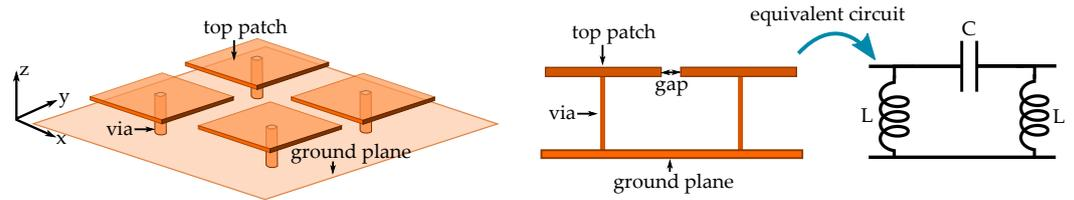
**Figure 2.** Sievenpiper mushroom-like metasurface and its equivalent electric circuit.
