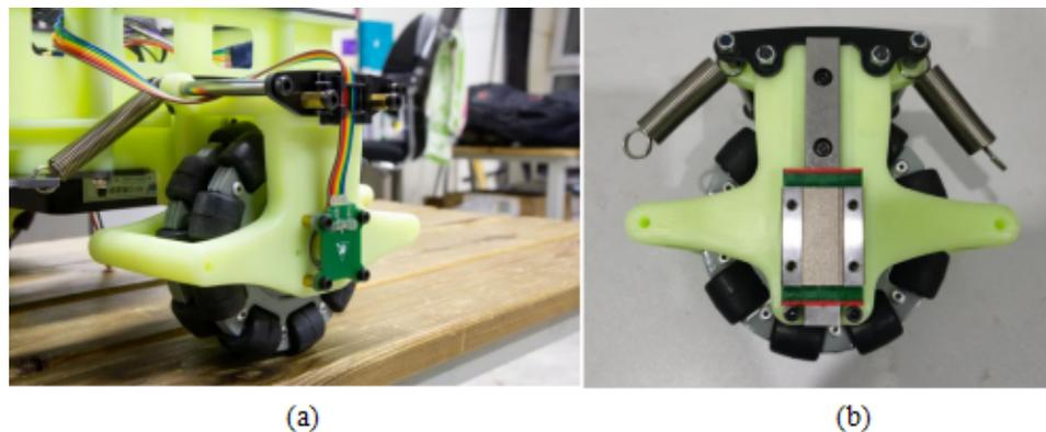
**Figure 2.** (a) Physical picture of encoder and slave wheel installation. (b) Physical drawing of sliding mechanism. The range of up and down movement is 6 cm. Every sliding mechanism supports the amount of ground unevenness at  $\pm 3$  cm.
