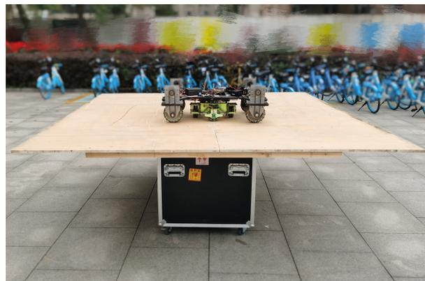
**Figure 23.** Simulation floating experimental platform, size of 2.4 m × 2.4 m.
