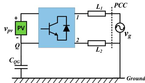
Figure 1. Typical single-phase grid-connected PV converter.
