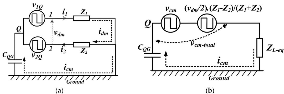
**Figure 2.** (a) Common-mode equivalent circuit of single-phase grid-connected converter, (b) simplified equivalent circuit for the total common-mode voltage.
