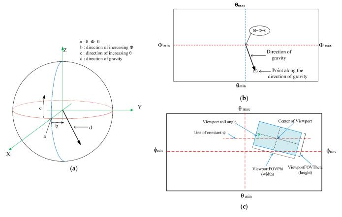
**Figure 4.** Graphical overview of ERP image: (**a**) spherical and cartesian coordinates, (**b**) generalized description of ERP mapped on 2D plane, and (**c**) generalized description of the viewport.
