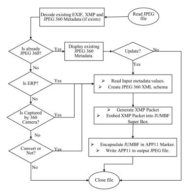
Figure 6. Workflow of the proposed JPEG 360 converter.
