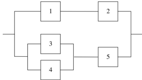
Figure 2. The network with series and parallel elements.
