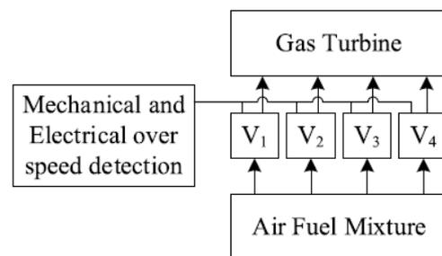
Figure 4. The overspeed protection of a gas turbine system.
