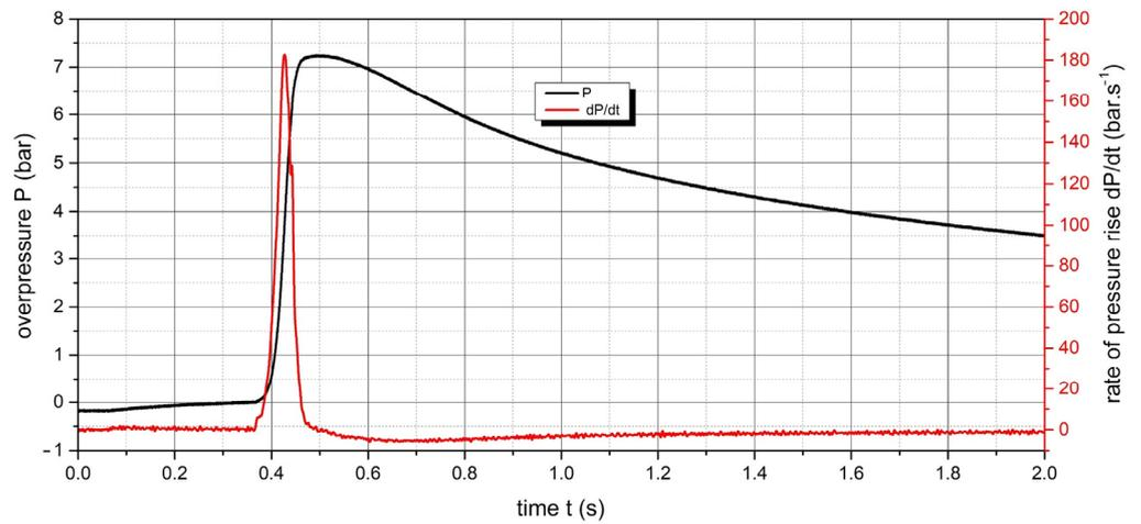
Figure 6. Overpressure P and rate of pressure rise  $dP/dt$  of  $250 \text{ g}\cdot\text{m}^{-3}$  *Lycopodium clavatum* powder ignited by Igniter 1 (shelf life less than 1 year).
