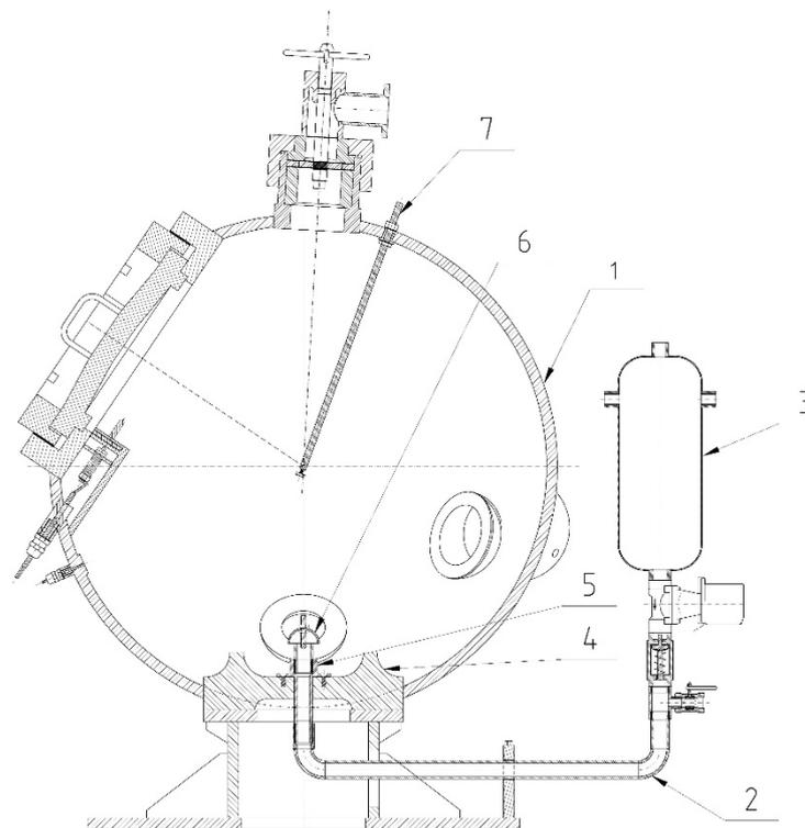
**Figure 1.** Cross section of 365 L explosion chamber (1—explosion spherical chamber, 2—disperser tube, 3—pressure vessel, 4—dispersing plate, 5, 6—disperser, 7—igniter rod) (Reprinted Ref. [25]).
