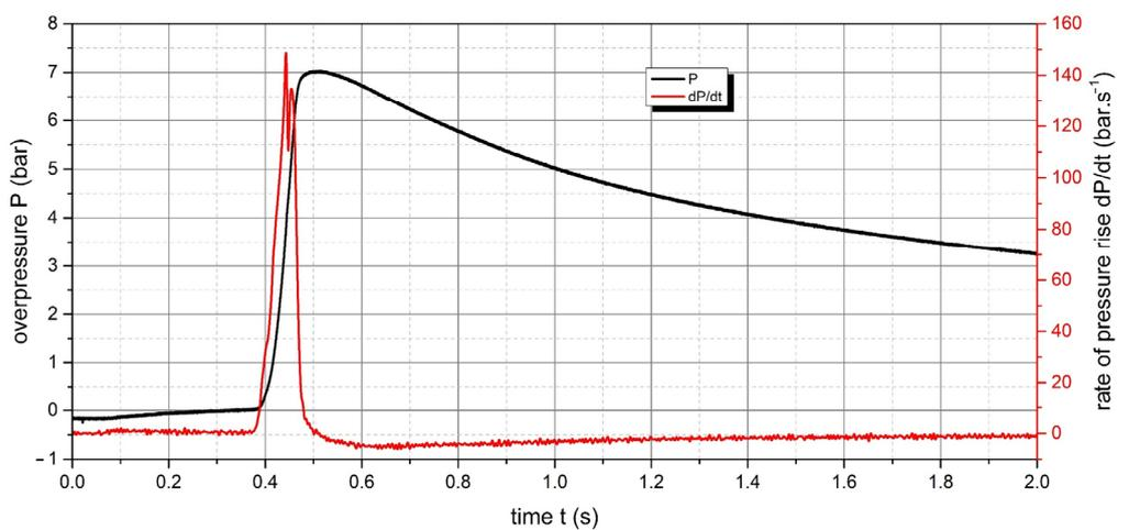
Figure 7. Overpressure P and rate of pressure rise  $dP/dt$  of  $250 \text{ g}\cdot\text{m}^{-3}$  *Lycopodium clavatum* powder ignited by Igniter 2 (shelf life more than 2 years).
