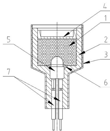
**Figure 4.** Cross section of commercially available igniter (redrawn according to patent application Chemical detonator with electric trigger—US 2016/0102957 A1 [27]) 1—pyrotechnic composition filling, 2—plastic case, 3—metal case, 4—stopper, 5—fuse head, 6—fuse head sealing, 7—priming wires.
