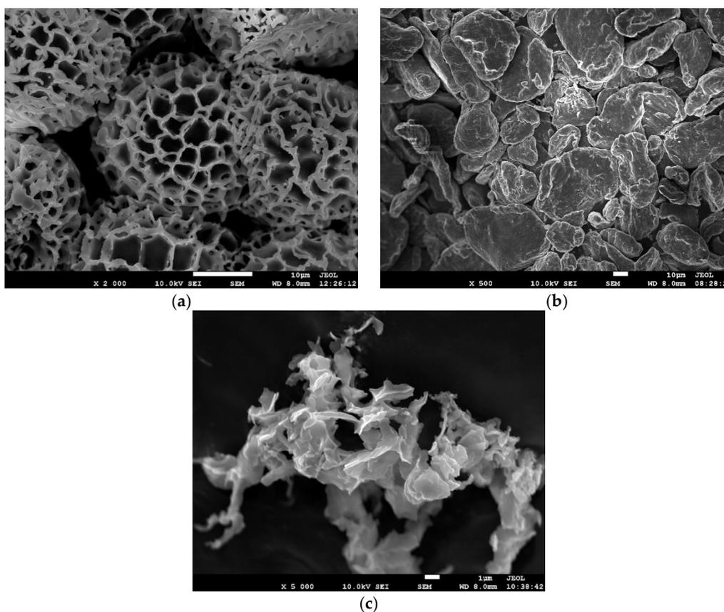
Figure 3. Microstructure of the samples (SEM). (a) *Lycopodium clavatum* powder particles, (b) Magnesium powder particles, (c) Benzoic acid sample.
