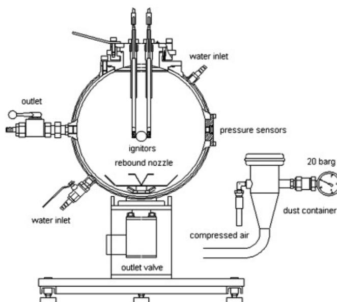
Figure 2. 20 L apparatus (Kühner AG) (Reprinted Ref. [26]).
