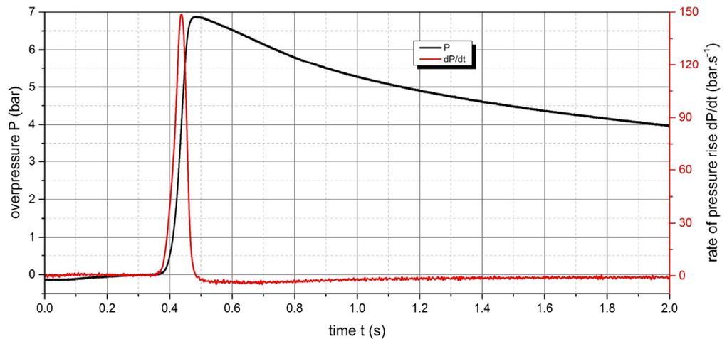
**Figure 9.** Overpressure  $P$  and rate of pressure rise  $dP/dt$  of  $500 \text{ g}\cdot\text{m}^{-3}$  *Lycopodium clavatum* powder ignited by Igniter 2 (shelf life 2 years).
