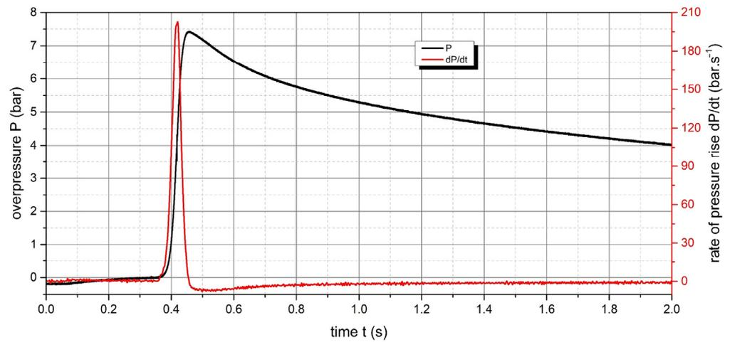
**Figure 8.** Overpressure  $P$  and rate of pressure rise  $dP/dt$  of  $500 \text{ g}\cdot\text{m}^{-3}$  *Lycopodium clavatum* powder ignited by Igniter 1 (shelf life less than 1 year).
