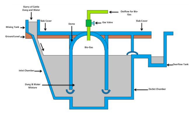
Figure 6. Fixed dome types of biogas plants in India.
