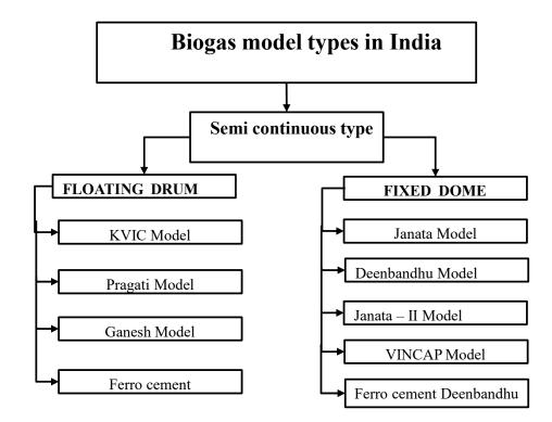
Figure 4. Classification of various types of biogas plants in India.
