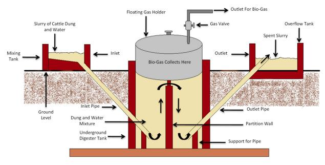
Figure 5. Floating dome types of biogas plants in India.
