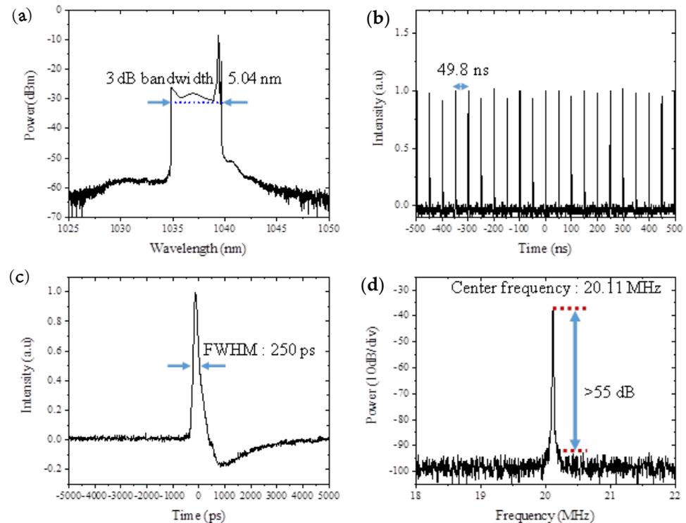
**Figure 5.** Characteristics of the 1  $\mu\text{m}$  mode-locked pulse laser at a pump power of 247 mW: (a) optical spectrum; (b) oscilloscope trace; (c) high-speed oscilloscope trace and estimated pulse duration; (d) RF spectrum.
