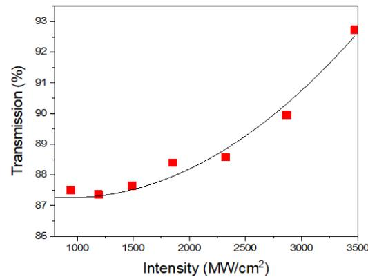
**Figure 2.** Nonlinear transmission measurement of the DNA SA at a wavelength of 1550 nm.
