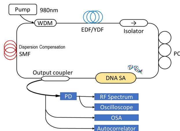
**Figure 3.** Experimental setup of the passively mode-locked fiber laser using liquid DNA as the SA.
