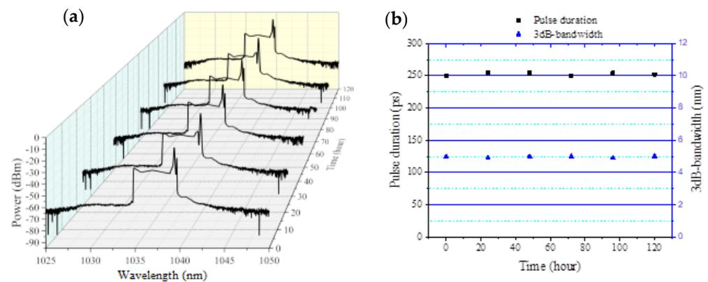
**Figure 6.** (a) Optical spectrum and pulse duration; (b) 3 dB bandwidth as a function of time.
