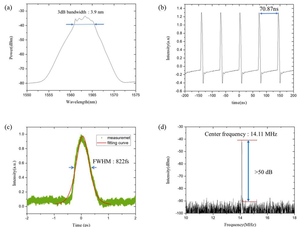
**Figure 4.** Soliton pulse train of the 1.5  $\mu\text{m}$  passively mode-locked fiber laser: (a) optical spectrum; (b) oscilloscope trace; (c) autocorrelation trace; (d) RF spectrum.
