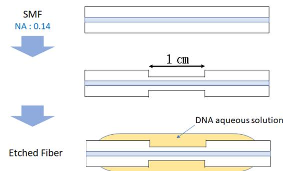
**Figure 1.** Fabrication process and cross-section of the DNA SA.
