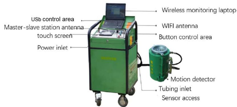
Figure 6. The feedback control system and supporting facilities.
