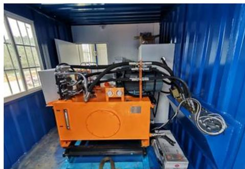
**Figure 15.** Workstation intelligent control hydraulic pump.
