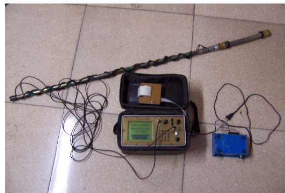
Figure 5. Phd-2 multifunctional ultrasonic detector.
