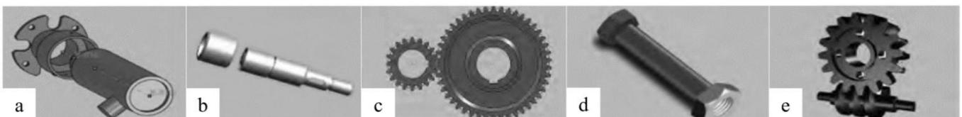
**Figure 3.** The types of typical assembly tasks: (a) matching, (b) conjugating, (c) joining, (d) fastening, and (e) meshing.
