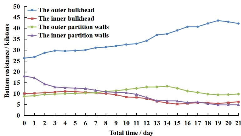
Figure 19. Variation curves of end resistance in different area by field data.
