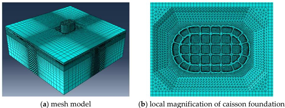
Figure 10. Finite element mesh model.
