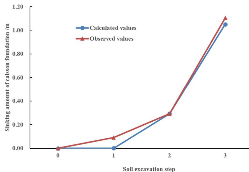
Figure 15. Sinking amount comparison between numerical results and the field measurements.
