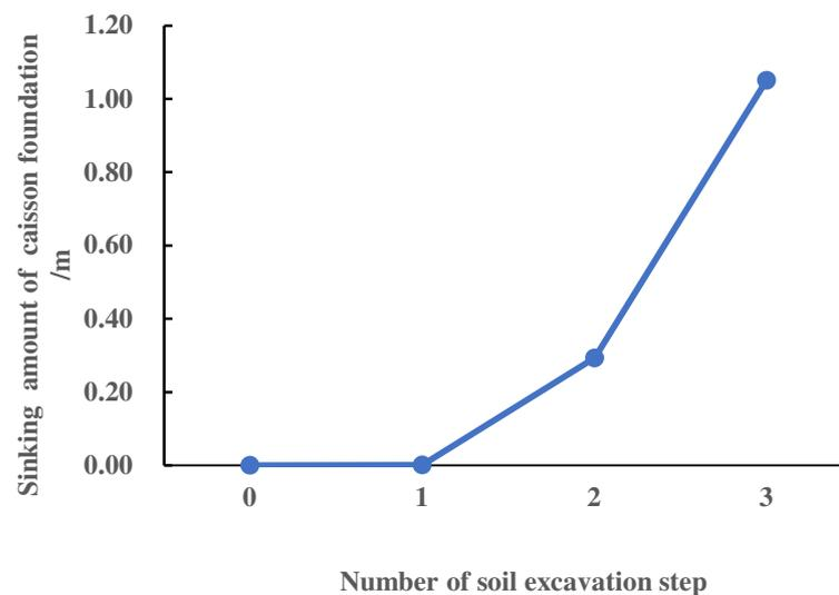
Figure 11. Sinking amount corresponding to the step of soil excavation.
