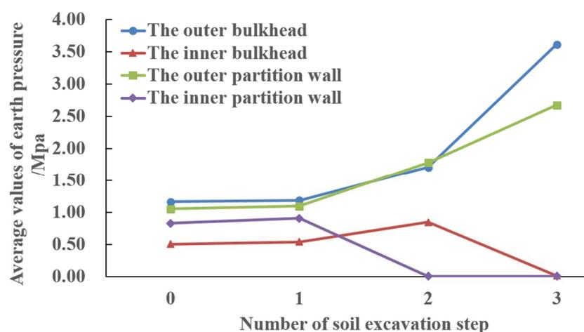
**Figure 14.** Average earth pressure with soil excavation step by numerical analysis.
