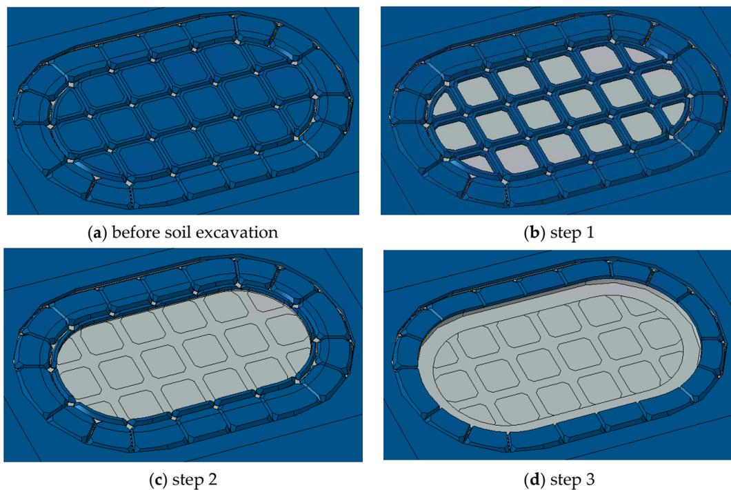
**Figure 8.** Schematic diagram of soil excavation steps at the first stage.
