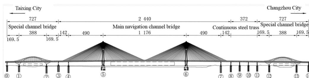
Figure 1. Main Bridge of Changtai Yangtze River Bridge.
