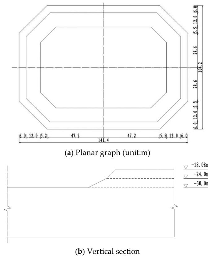
**Figure 4.** Schematic diagram of underwater slope.
