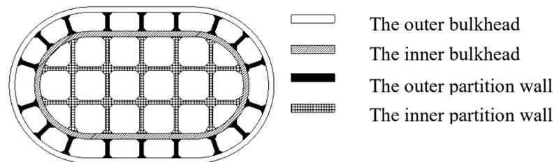
Figure 3. Different area at the bottom of caisson foundation.
