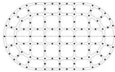
**Figure 5.** Layout of soil pressure sensors.
