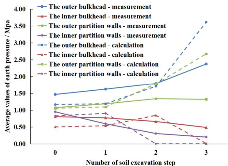
Figure 20. Comparison of earth pressure with soil excavation step.
