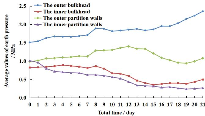
Figure 17. Variation curves of average measured earth pressure.
