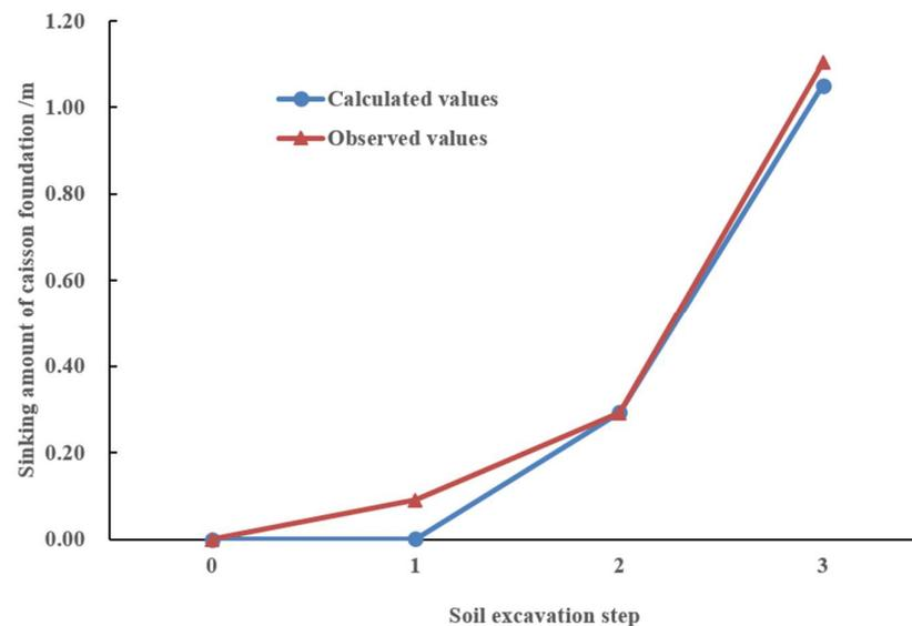
Figure 15. Sinking amount comparison between numerical results and the field measurements.
