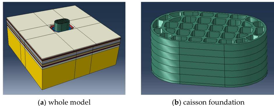
Figure 9. 3-D Finite element model.
