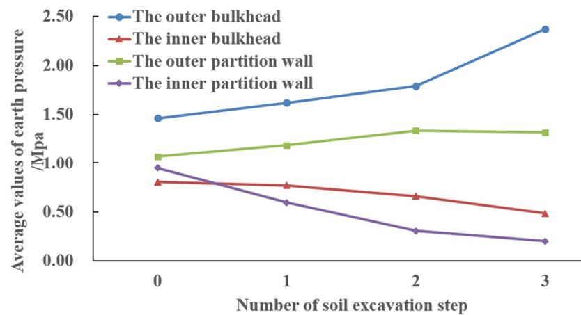
**Figure 18.** Averages of the field measured soil pressure with soil excavation step.
