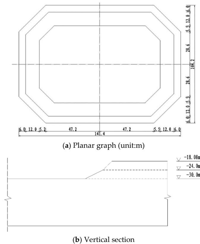
**Figure 4.** Schematic diagram of underwater slope.
