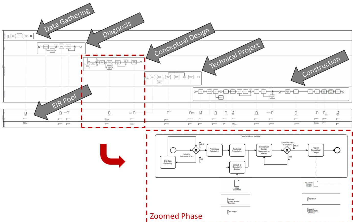
**Figure 9.** Specific façade renovation BPMN diagram (ID2, architect). The conceptual design phase is zoomed.
