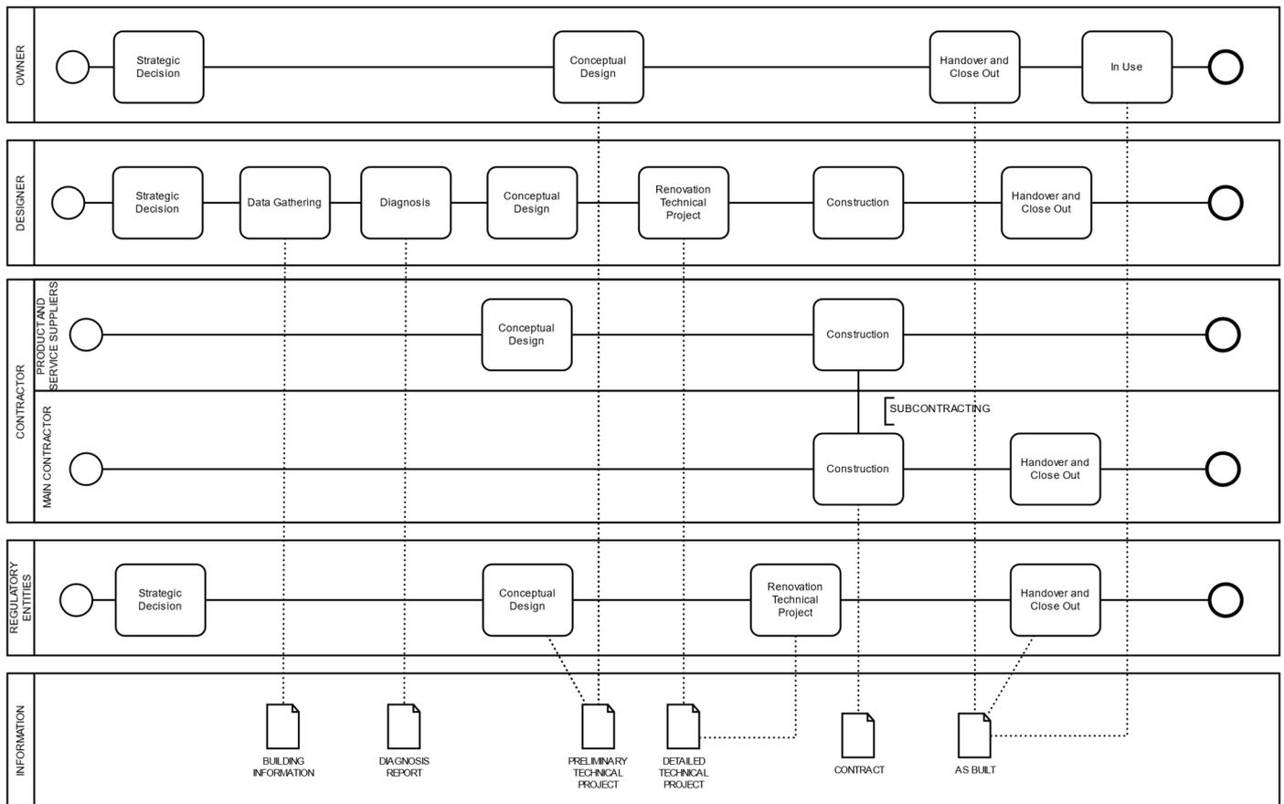
**Figure 8.** Generic renovation process represented in a BPMN diagram (ID1).
