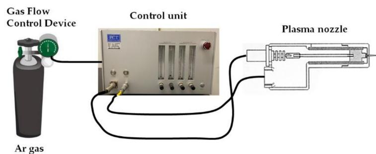
**Figure 1.** Argon-based non-thermal atmospheric pressure plasma (NTAPP) stimulation device used in this study. The multi-gas plasma jet source has a columnar body like a pen connected to an AC power supply of 16 kHz and 9 kV and a gas cylinder.
