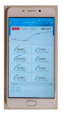
Figure 10. Internet of things measurement system—mobile terminal.
