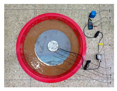
**Figure 7.** Ground pressure calibration device. 1. 12 V power supply. 2. Arduino controller. 3. Wireless serial port transceiver module. 4. Signal amplifier. 5. Pressure sensor. 6. Mounting base. 7. Counterweight plate. 8. Bottom plate.
