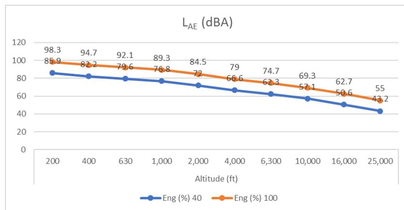
Figure 34. NPD curves, in terms of L<sub>AE</sub>, for the DEP configuration.
