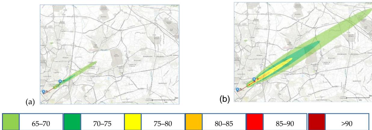
**Figure 41.** Graphical representation of equal loudness contours for the conventional (a) and hybrid (b) configurations, in terms of  $L_{AE}$  (dB-A), for a standard runway-24 landing.
