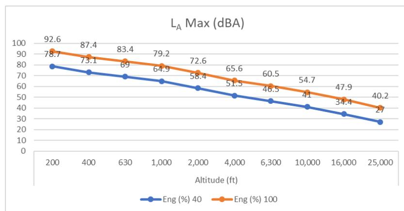
Figure 35. NPD curves, in terms of L<sub>A</sub>Max, for the DEP configuration.
