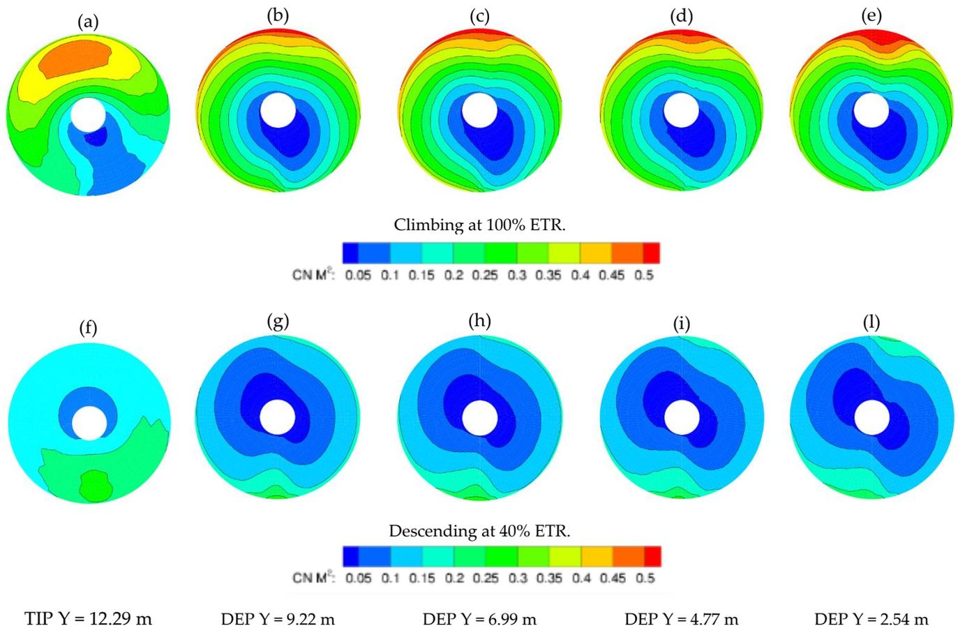
Figure 17. Motorization2 -  $CN M^2$  distribution on the propellers' disks, starboard side. From (a) to (e), load on the disk from Tip to inner propellers, in Climb condition. From (f) to (l), same results in Descent flight.
