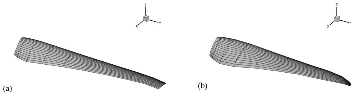
**Figure 9.** Rotor blades' discretized geometry. Tip propeller (a); DEP propellers (b).
