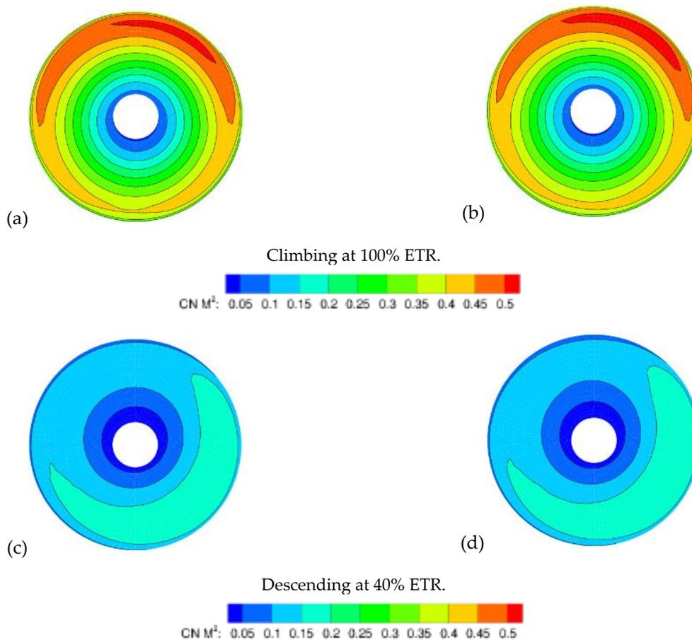
Figure 14. Configuration A –  $CN M^2$  distribution on propellers' disks. Starboard side (a and c); portside (b and d), in the two cases of Climbing (a and b) and Descent (c and d) flight.
