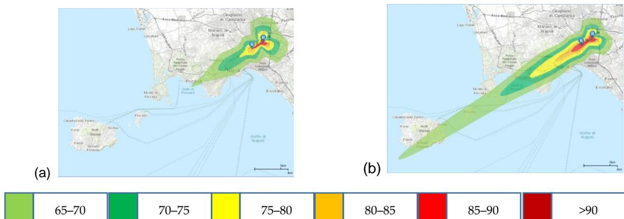
**Figure 39.** Graphical representation of equal loudness contours for the conventional (a) and hybrid (b) configurations, in terms of  $L_{Ae}$ (dB-A), for a standard runway-24 take-off.
