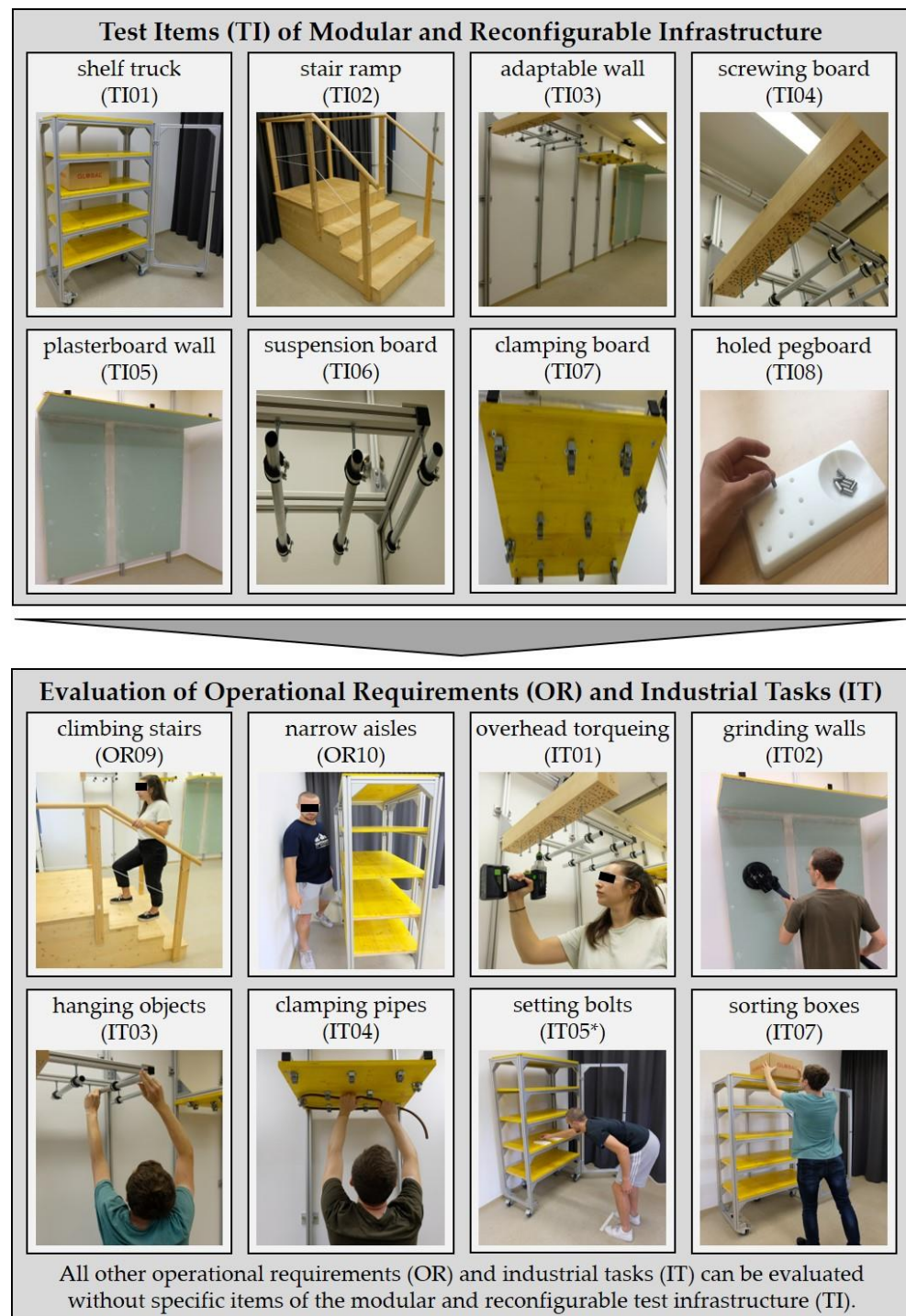
Figure 4. Items of test course infrastructure with exemplary arrangements and applications for the evaluation of operational requirements and industrial tasks (baseline scenario).
