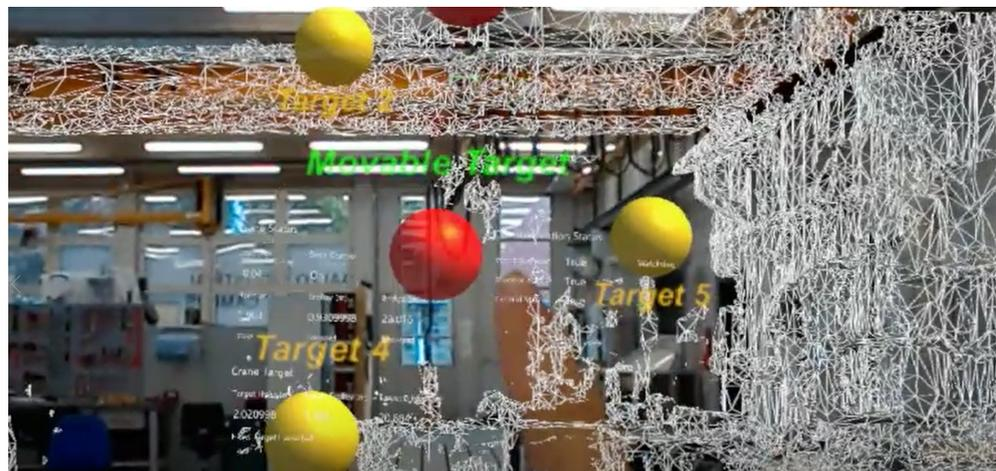
**Figure 4.** HoloLens view while the user was navigating the movable target: the spatial mapping mesh of the AIIC space captured by the HoloLens camera was also displayed in the scene, to enhance users’ spatial awareness and reduce the risk of placing the movable target in inaccessible locations.
