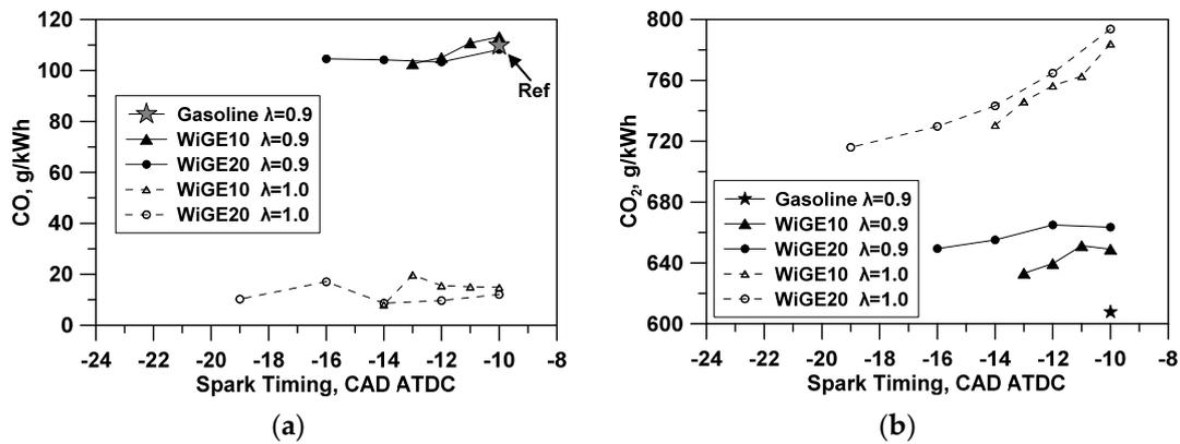
Figure 6. CO (a) and CO<sub>2</sub> (b) emissions against spark timing and relative air-to-fuel ratio.
