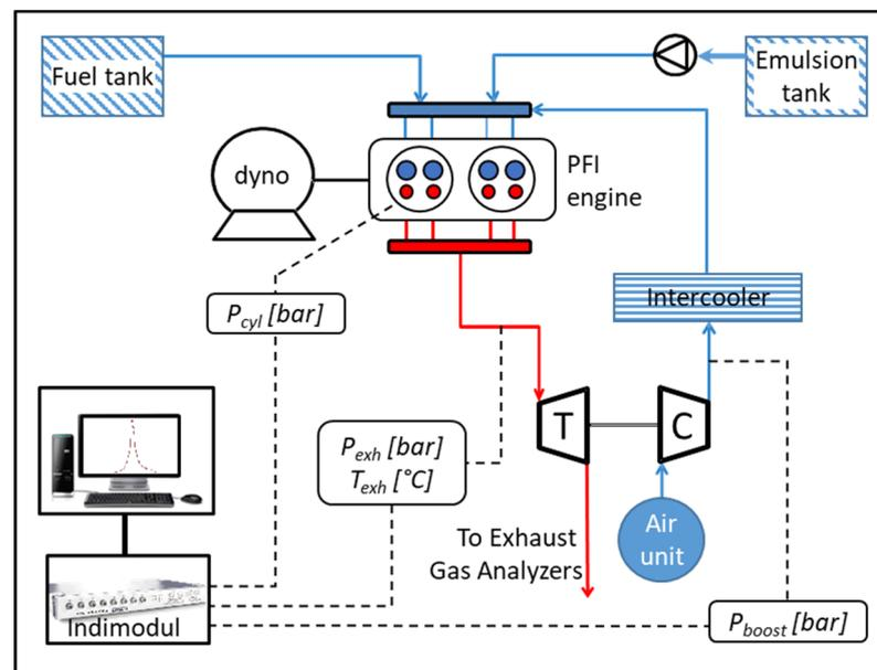
Figure 1. General layout of the experimental setup.
