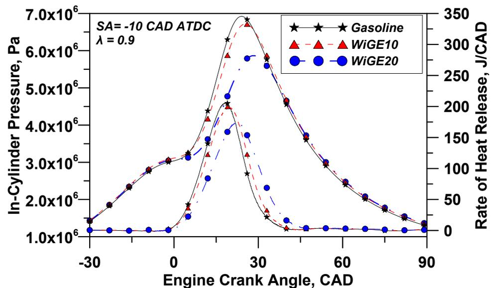
Figure 2. In-cylinder pressure trace and rate of heat release at SA =  $-10$  CAD ATDC,  $\lambda = 0.9$ .
