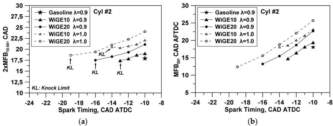
Figure 3. Combustion duration ( $2 \times MFB_{10-50}$ ) (a) and combustion center ( $MFB_{50}$ ) (b) against spark timing and relative air-to-fuel ratio for WiGE 10 and WiGE 20.
