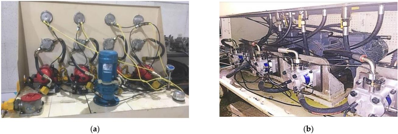
Figure 3. Life-cycle test bed of gear pump: (a) Topside of test bed and (b) Underside of test bed.
