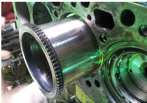
**Figure 6.** Rotating liner pulled a few inches out of the block, exposing the outside surface.
