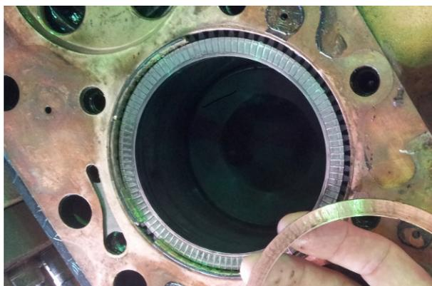
**Figure 5.** Details of the rotating liner face seal features. The copper head gasket only needs to seal oil and coolant. This picture is shown again in the Appendix A with a higher resolution.
