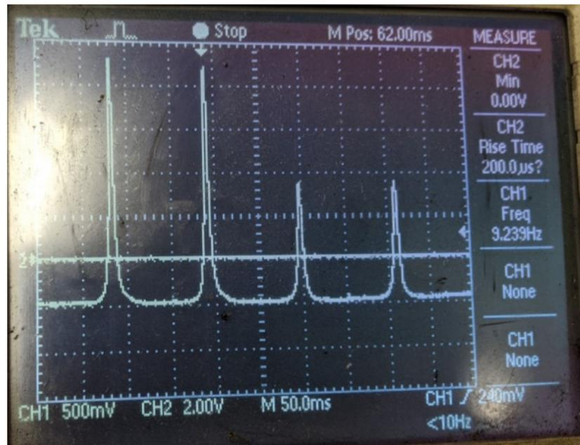
**Figure A3.** Motoring test on the BS, establishing its motoring pressure. The engine is revved up and the injection pump is turned off. As the engine continues to rotate, we record the peak pressure. Each division is 10 bar. The x axis scale gives us the speed estimate. The speed here is about 1050 rpm. The peak pressure will drop slightly to 750 rpm, but we are using this figure of about 27 bar gage or 28 bar absolute.
