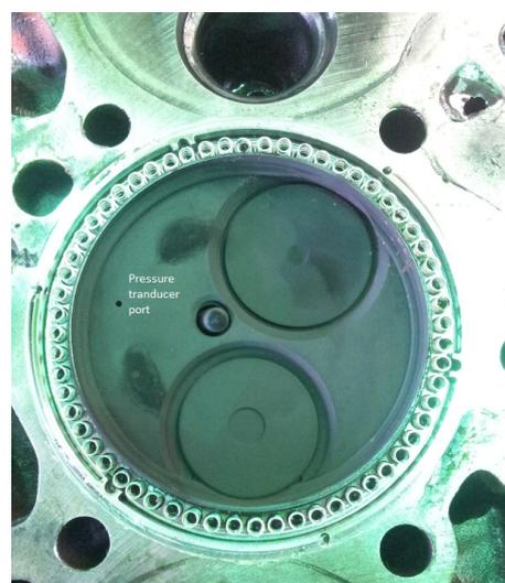
**Figure A2.** Detail of the cylinder head modification. Note that the seal gland area is completely free from carbon deposits.
