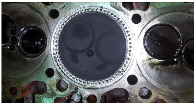
**Figure 7.** Cylinder head, showing the head insert that houses the primary sealing ring, springs that pre-load the primary sealing ring, and secondary seal.
