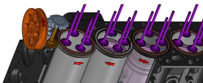
**Figure 17.** CAD representation of the multi-cylinder RLE. The critical components are identical to the current prototype, and the model of the block is the production engine, so a direct modification is feasible.
