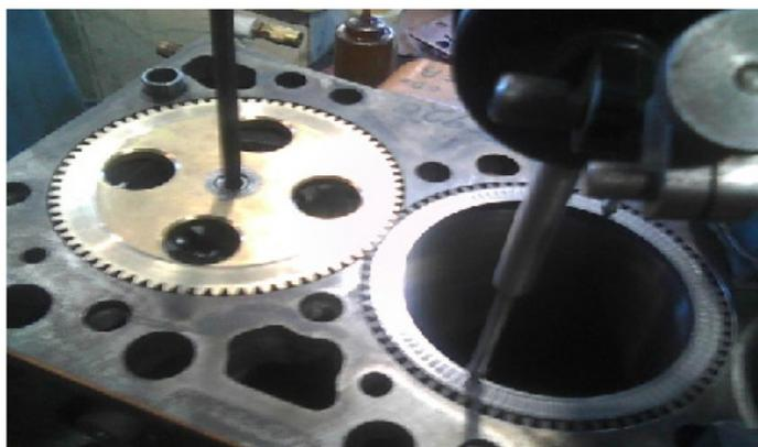
**Figure 4.** Block of the RLE diesel prototype. The driving gear could be replaced by another rotating liner, so the engine could operate as a complete four-cylinder 4BT RLE.
