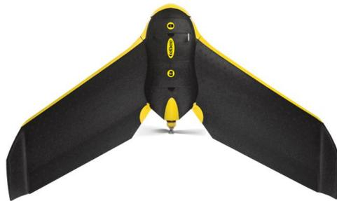
**Figure 5.** The Remotely piloted aircraft system (RPAS) eBee.
