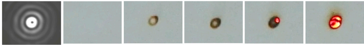
Figure 3. Image of a quasi-Bessel beam formed with a binary axicon and recorded by a microbolometer detector array (compare with Figure 1e). Right: sequence of video frames demonstrating firing paper with this beam. In this case, no polarization converter was used, and the beam had linear polarization. Frame dimensions were 16.32 \times 12.24 \text{ mm}^2 .
