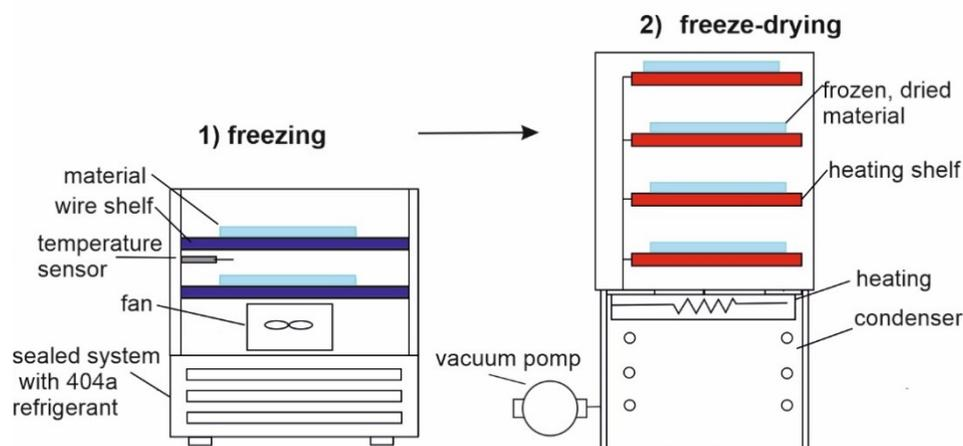
**Figure 1.** Scheme of lyophilization equipment.
