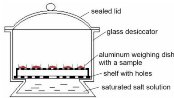
Figure 2. Sorption isotherms—the experimental set up of static method.
