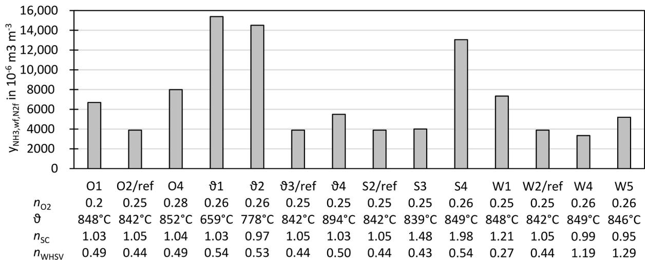
Figure 16. Compilation of all conducted NH<sub>3</sub> measurements.
