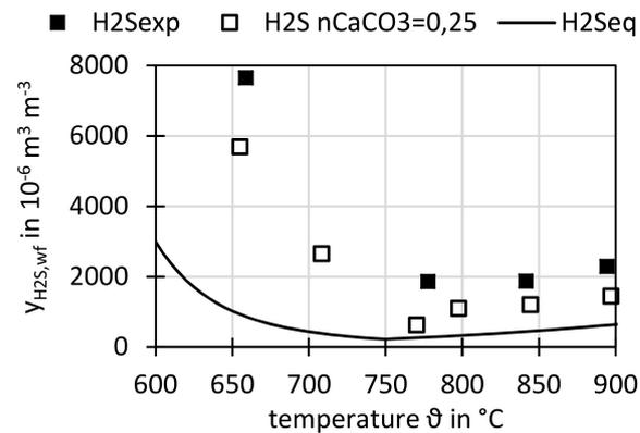
**Figure 12.** Measured and equilibrium H<sub>2</sub>S concentration on dry and N<sub>2</sub>-free basis at different temperatures  $\vartheta$ .
