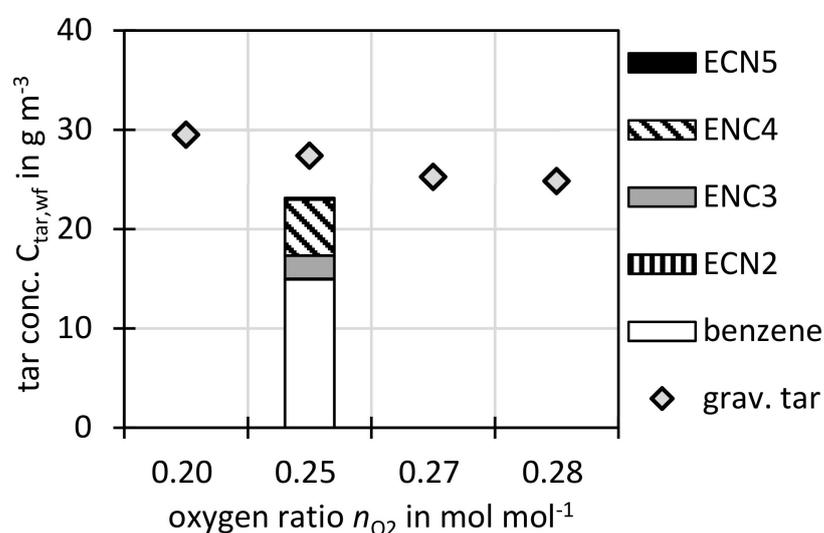
**Figure 6.** Gravimetric and GC tar concentrations dry, N<sub>2</sub>-free and STP basis at different oxygen ratios  $n_{O_2}$  and constant  $\vartheta$ .
