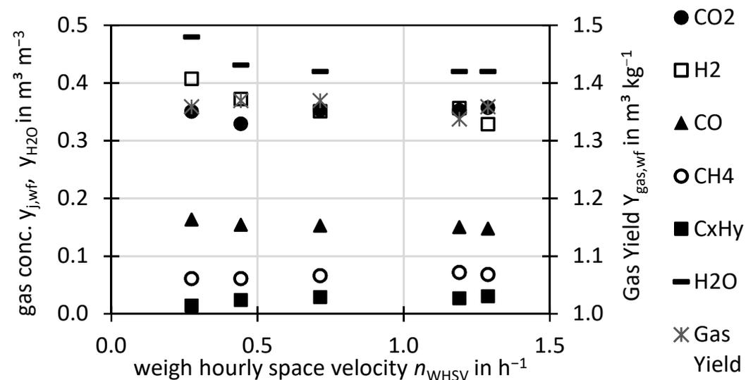
**Figure 5.** Permanent gas concentrations for different  $n_{WHSV}$  in dry N<sub>2</sub>-free basis, for H<sub>2</sub>O wet N<sub>2</sub>-free basis and dry N<sub>2</sub>-free gas yield per dry ash free fuel.
