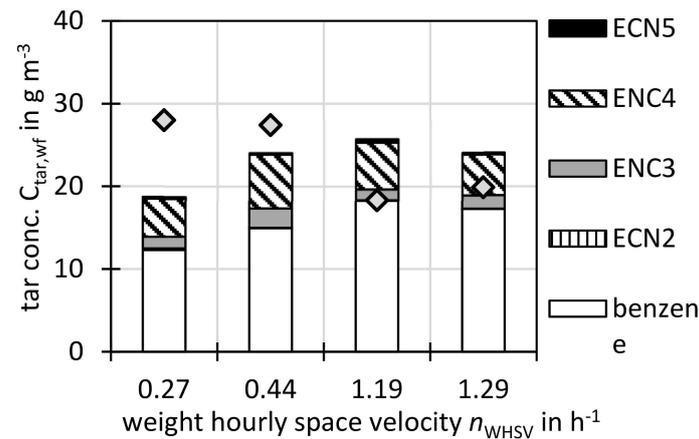
**Figure 9.** Gravimetric and GC-MS tar concentrations on dry, N<sub>2</sub>-free and STP basis at different weight hourly space velocities.
