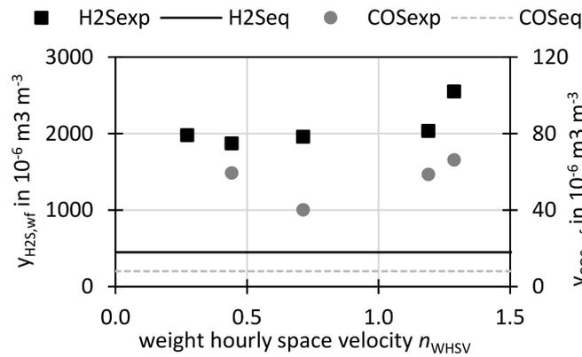
Figure 15. Measured and equilibrium H<sub>2</sub>S and COS concentration at different fuel space velocities.
