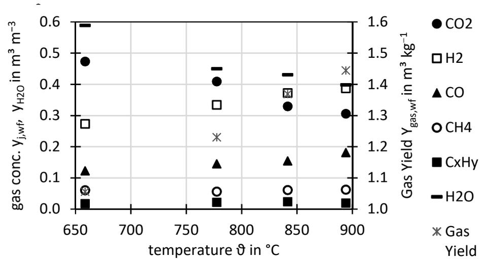
Figure 3. Permanent gas concentrations in dry N<sub>2</sub>-free basis, for H<sub>2</sub>O wet N<sub>2</sub>-free basis and dry N<sub>2</sub>-free gas yield per dry ash free fuel for different temperatures  $\vartheta$  at constant  $n_{O_2}$ .
