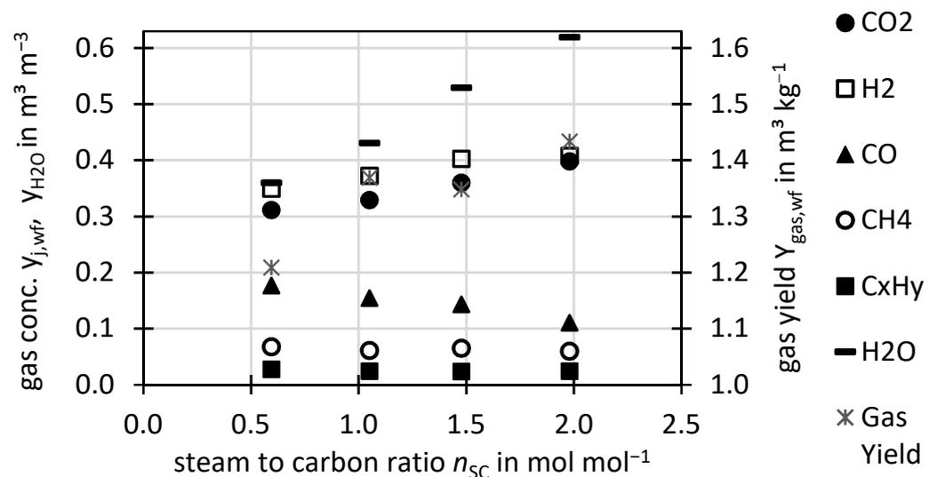
Figure 4. Permanent gas concentrations for different  $n_{SC}$  in dry N<sub>2</sub>-free basis, for H<sub>2</sub>O wet N<sub>2</sub>-free basis and dry N<sub>2</sub>-free gas yield per dry ash free fuel.
