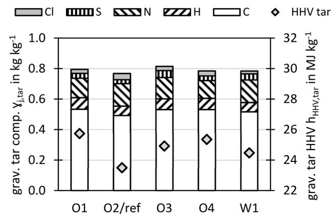
**Figure 10.** Elemental analysis and heating values of gravimetric tars.
