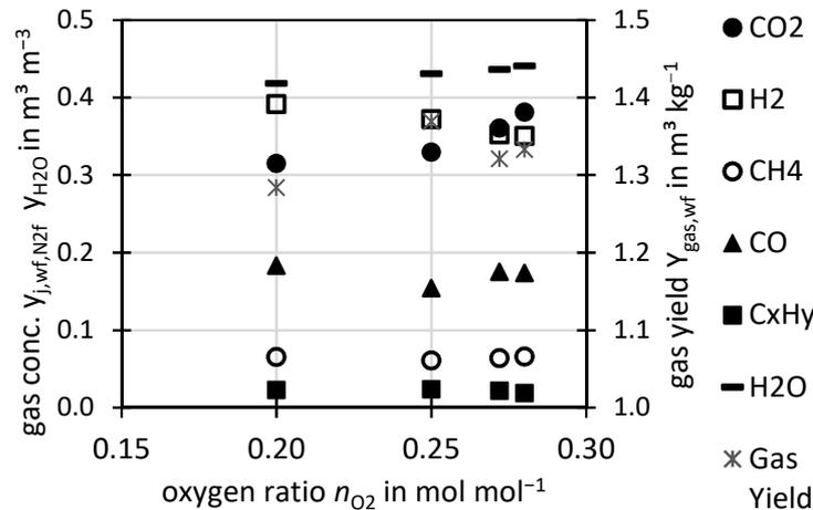
**Figure 2.** Permanent gas concentrations in dry  $N_2$ -free basis, for  $H_2O$  wet  $N_2$ -free basis and dry  $N_2$ -free gas yield per dry ash free fuel at different oxygen ratios  $n_{O_2}$  and constant  $\vartheta$ .
