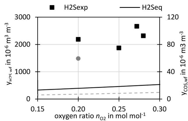
**Figure 11.** Measured and equilibrium H<sub>2</sub>S and COS concentrations on dry and N<sub>2</sub>-free basis at different oxygen ratios  $n_{O_2}$  and constant  $\vartheta$ .
