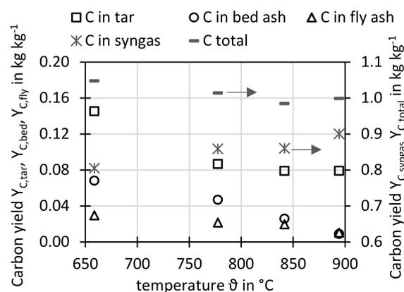
**Figure 17.** Carbon balance: Yield of carbon in syngas, tar, bed ash, fly ash and total sum for different gasifier temperatures.
