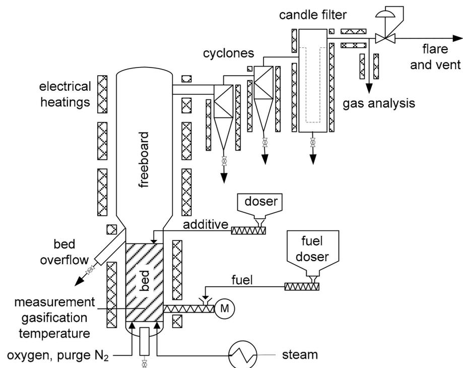
**Figure 1.** 20 kW fluidized bed gasification facility.
