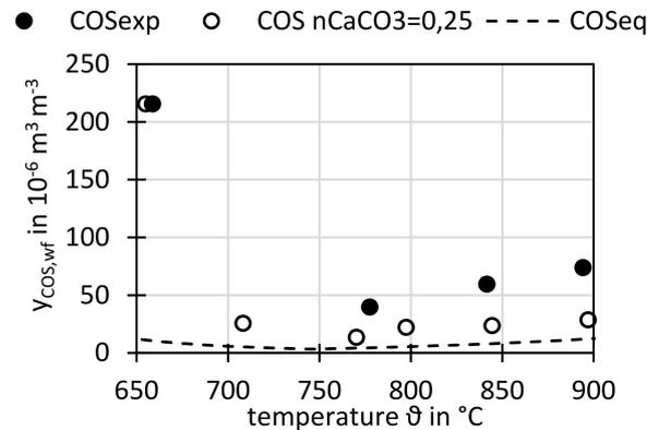
**Figure 13.** Measured and equilibrium COS concentration on dry and N<sub>2</sub>-free basis at different temperatures  $\vartheta$ .
