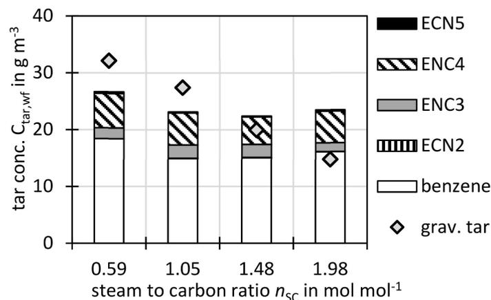
**Figure 8.** Gravimetric and GC tar concentrations on dry, N<sub>2</sub>-free and STP basis at different steam to carbon ratios  $n_{SC}$ .
