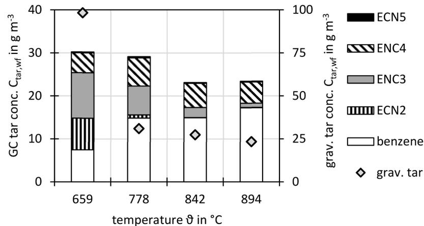
**Figure 7.** Gravimetric and GC tar concentrations on dry, N<sub>2</sub>-free and STP basis at different gasifier temperatures.
