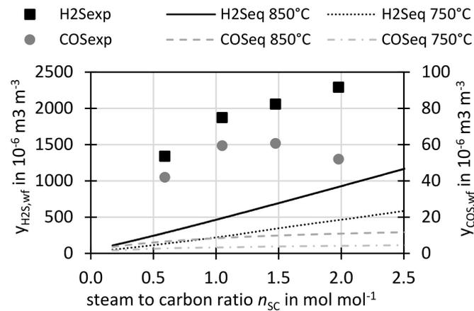
**Figure 14.** Measured and equilibrium  $H_2S$  and  $COS$  concentration on dry and  $N_2$ -free basis at different steam to carbon ratios, additionally equilibrium calculations for  $\vartheta = 750 \text{ }^\circ\text{C}$  are showing the best possible sulfur capture.
