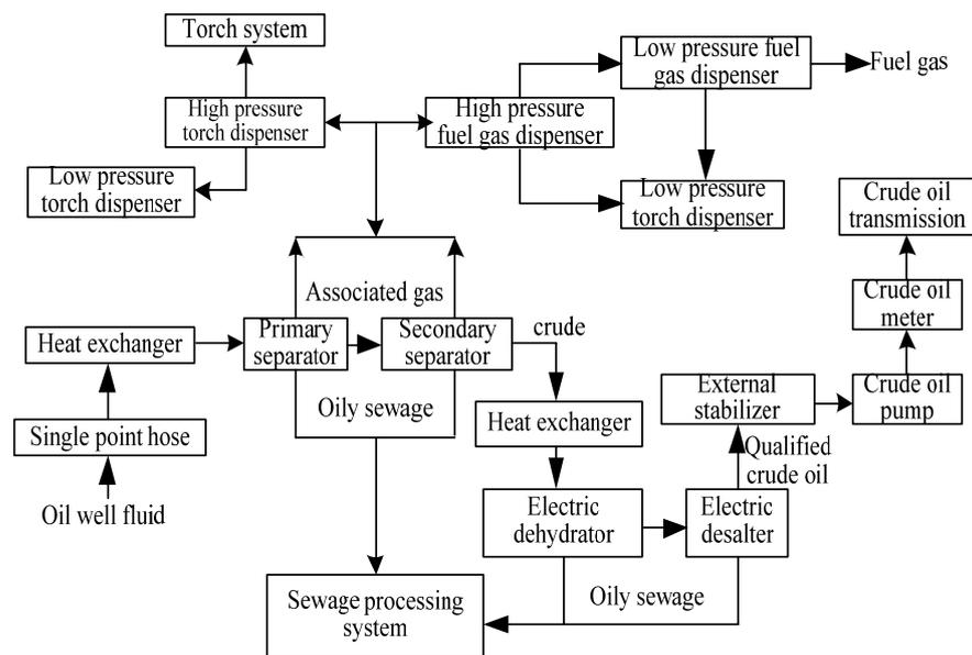
**Figure 1.** The processing technology flow diagram of floating production storage and offloading system (FPSO) oil and gas processing system.
