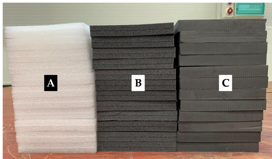
**Figure 3.** Samples used in this study. (A) PE25, (B) PE30, and (C) XPE.
