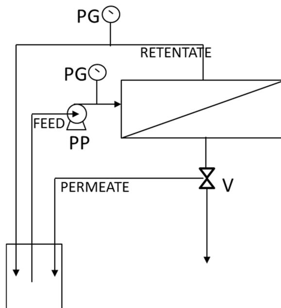
**Figure 1.** Schematic representation of cross-flow ultrafiltration system used. PG: pressure gauges, PP: peristaltic pump, V: valve. The same system was used to work in recycle mode (recirculating the permeate) and in concentration mode.
