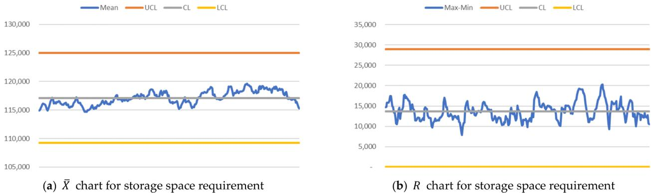
**Figure 6.**  $\bar{X} - R$  charts over time-shifts (x-axis) for storage space requirement (y-axis) when trans-shipment and nontrans-shipment (inbound and outbound) TEUs are 80% and 20%, respectively, and 60% of arrived TEUs are transferred to other terminals.
