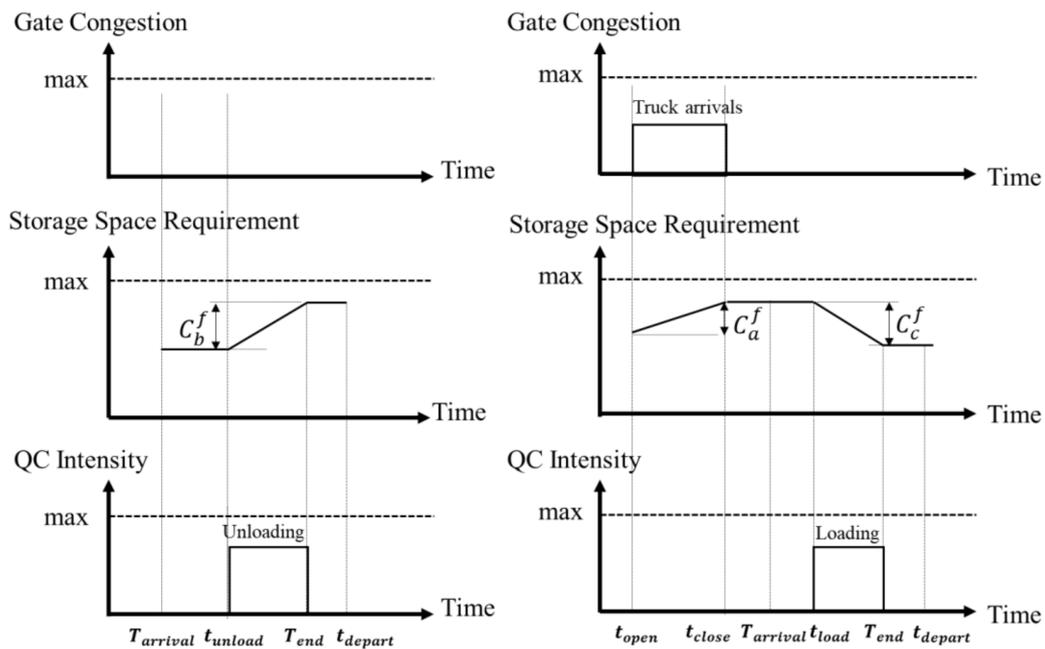
**Figure 2.** Simplified illustration of resource profiles for unloading (left) and loading (right) operations for a feeder vessel.
