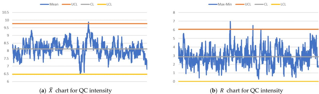
**Figure 5.**  $\bar{X} - R$  charts over time-shifts (x-axis) for QC intensity (y-axis) when trans-shipment and nontrans-shipment (inbound and outbound) TEUs are 80% and 20%, respectively, and 60% of arrived TEUs are transferred to other terminals.
