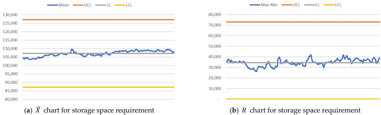
**Figure 9.**  $\bar{X} - R$  charts over time-shifts (x-axis) for storage space requirement (y-axis) when trans-shipment and nontrans-shipment (inbound and outbound) TEUs are 80% and 20%, respectively, and 75% of arrived TEUs are transferred to other terminals.
