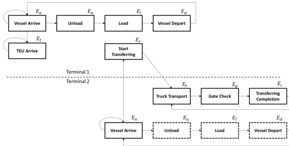
Figure 4. Event entity diagram for resource profile simulation.
