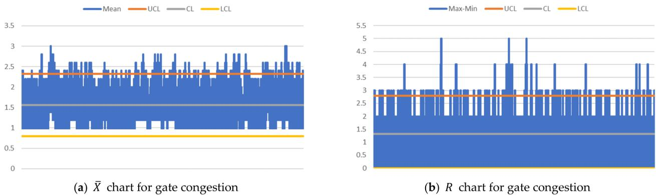
**Figure 7.**  $\bar{X} - R$  charts over time-shifts (x-axis) for gate congestion (truck queue) (y-axis) when trans-shipment and nontrans-shipment (inbound and outbound) TEUs are 80% and 20%, respectively, and 60% of arrived TEUs are transferred to other terminals.
