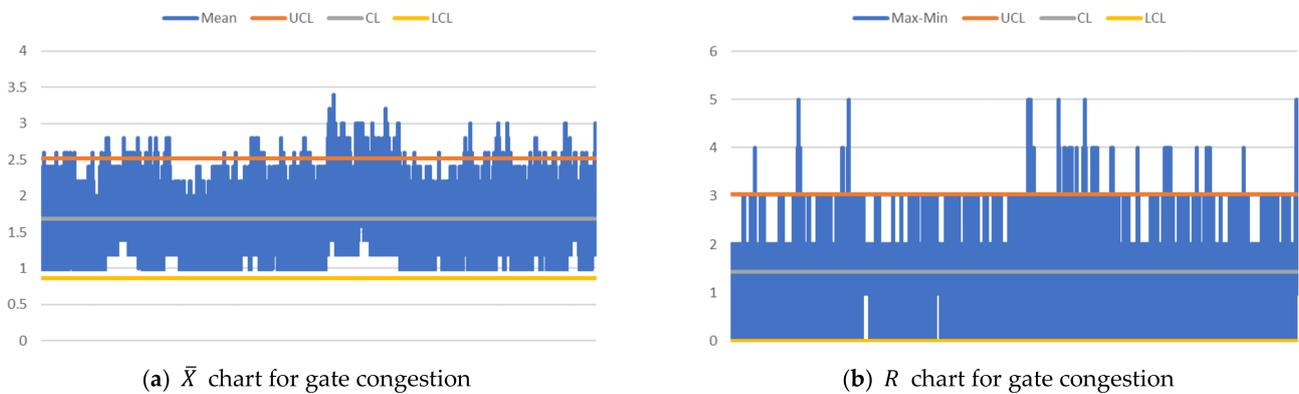
**Figure 10.**  $\bar{X} - R$  charts over time-shifts (x-axis) for gate congestion (truck queue) (y-axis) when trans-shipment and nontrans-shipment (inbound and outbound) TEUs are 80% and 20%, respectively, and 75% of arrived TEUs are transferred to other terminals.
