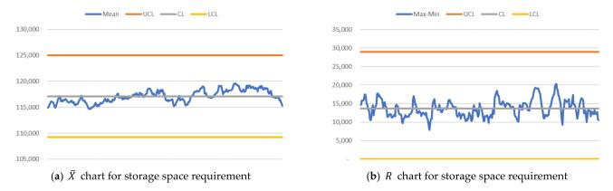
**Figure 6.**  $\overline{X}$  – R charts over time-shifts (x-axis) for storage space requirement (y-axis) when trans-shipment and nontrans-shipment (inbound and outbound) TEUs are 80% and 20%, respectively, and 60% of arrived TEUs are transferred to other terminals.
