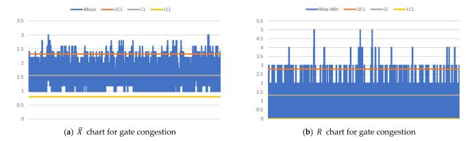
**Figure 7.**  $\overline{X}$  – R charts over time-shifts (x-axis) for gate congestion (truck queue) (y-axis) when trans-shipment and nontrans-shipment (inbound and outbound) TEUs are 80% and 20%, respectively, and 60% of arrived TEUs are transferred to other terminals.
