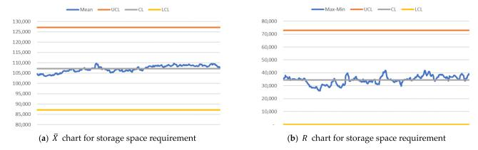
**Figure 9.**  $\overline{X} - R$  charts over time-shifts (x-axis) for storage space requirement (y-axis) when trans-shipment and nontrans-shipment (inbound and outbound) TEUs are 80% and 20%, respectively, and 75% of arrived TEUs are transferred to other terminals.
