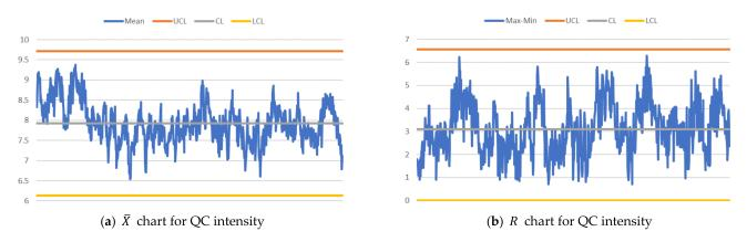
**Figure 8.**  $\overline{X} - R$  charts over time-shifts (x-axis) for QC intensity (y-axis) when trans-shipment and nontrans-shipment (inbound and outbound) TEUs are 80% and 20%, respectively, and 75% of arrived TEUs are transferred to other terminals.
