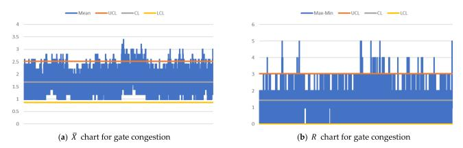
**Figure 10.**  $\overline{X}$  – R charts over time-shifts (x-axis) for gate congestion (truck queue) (y-axis) when trans-shipment and nontrans-shipment (inbound and outbound) TEUs are 80% and 20%, respectively, and 75% of arrived TEUs are transferred to other terminals.
