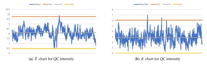
**Figure 5.**  $\overline{X} - R$  charts over time-shifts (x-axis) for QC intensity (y-axis) when trans-shipment and nontrans-shipment (inbound and outbound) TEUs are 80% and 20%, respectively, and 60% of arrived TEUs are transferred to other terminals.
