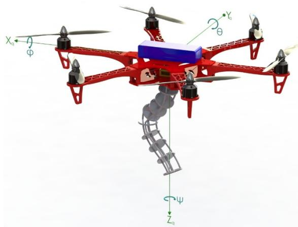
Figure 2. A hexa-rotor ACMS with a tendon-driven CR.
