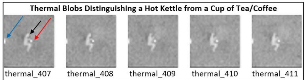
**Figure 5.** Distinguishable thermal blobs. On thermal\_407, the blue arrow points to the hot kettle, the black arrow points to the participant, and the red arrow to the tea/coffee cup after the initial act of tea/coffee making.
