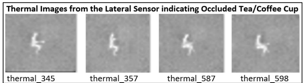
**Figure 6.** Thermal images from the lateral sensor indicating instances of occluded tea/coffee cups that are visible on the ceiling sensor. Refer to the thermal blobs with the same name as thermal\_345, thermal\_357, thermal\_587, and thermal\_598 in Figure 7.
