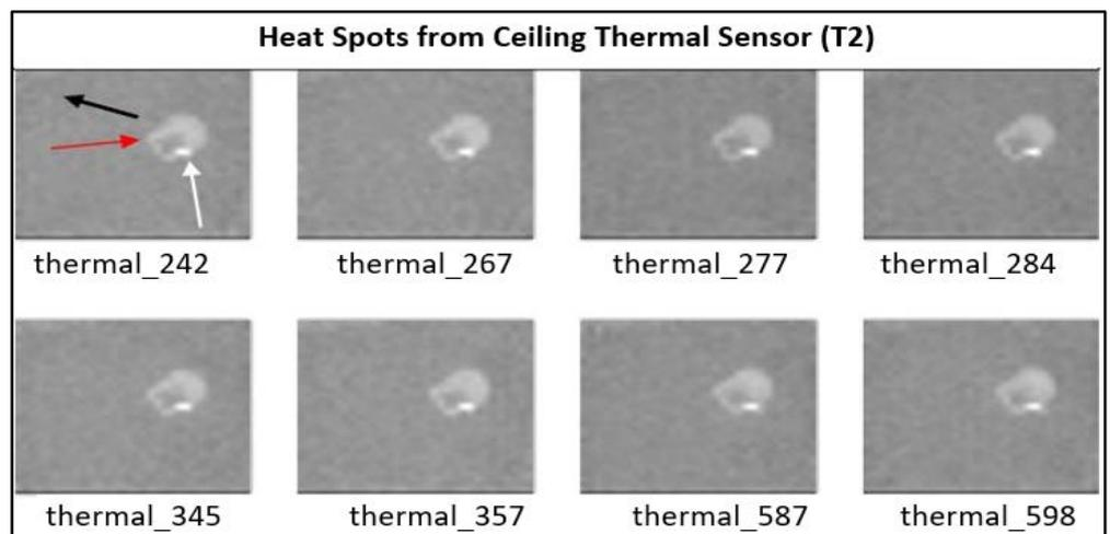
**Figure 7.** Heat pots from tea/coffee cups occluded from the lateral thermal sensor (T1) but indicated by the ceiling thermal sensor (T2). The black arrow on thermal\_242 points to the location of T1, the white arrow points to the heat spot, and the red arrow points to the hand of the participant (occluding the heat spot).
