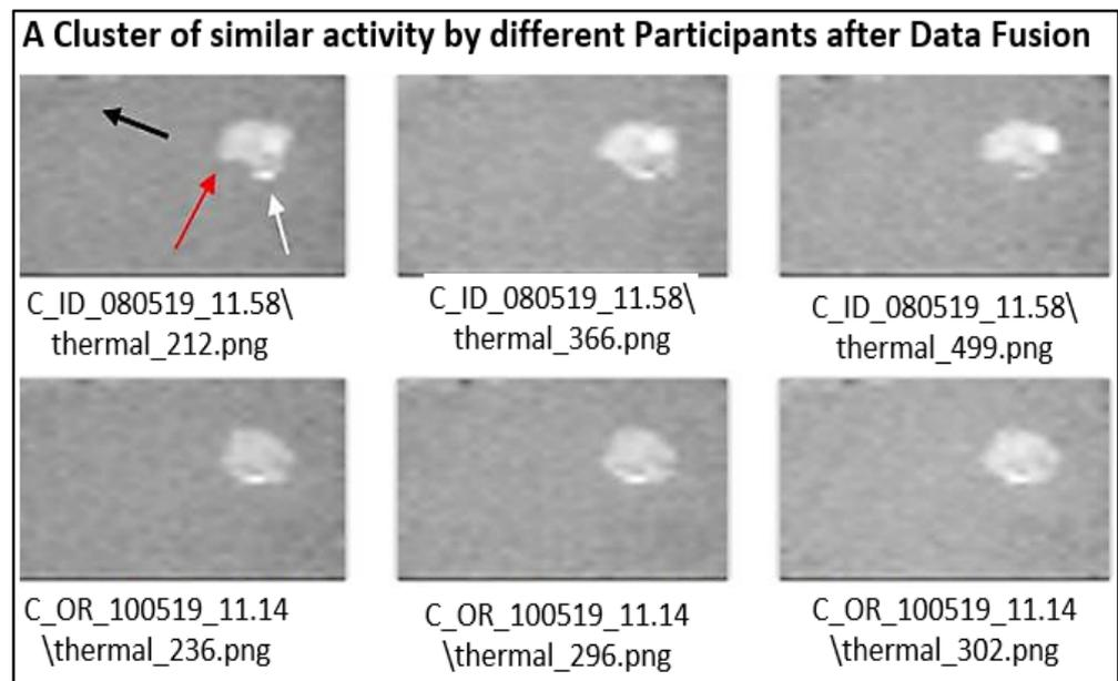
**Figure 9.** A cluster of data fusion output showing thermal blobs from two participants in a cluster with timestamps. The black arrow on ‘C\_ID\_080519\_11.58\thermal\_212.png’ points to the location of the lateral sensor, the red arrow points to the participant, and the white arrow points to the heat spot from tea/coffee cups.
