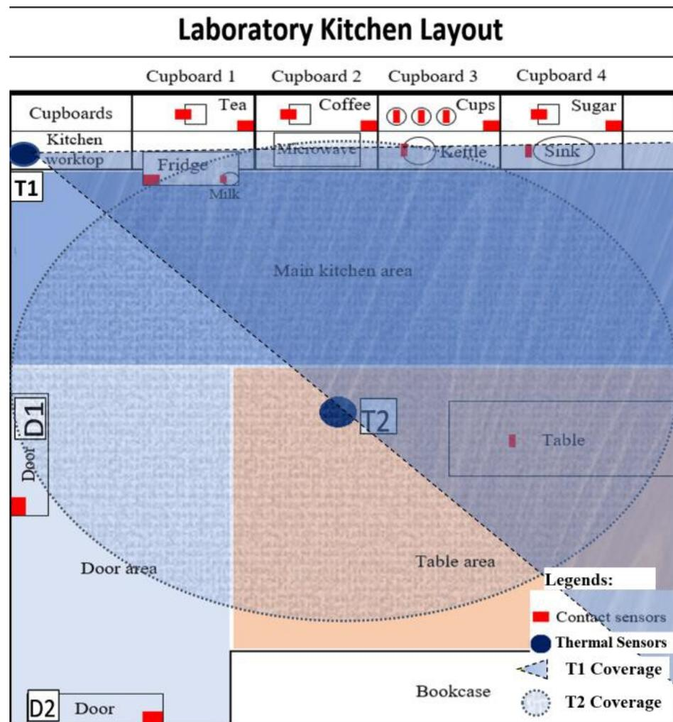
**Figure 2.** Laboratory kitchen layout. The areas marked in red indicate the location of the contact sensors. Thermal sensors are indicated by the navy-blue oval shape as T1 and T2 for lateral and ceiling thermal sensors, respectively. The coverage of T1 is indicated by the triangular area, while that of T2 is indicated by the oval area.
