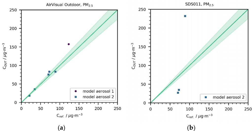
**Figure 4.**  $\text{PM}_{2.5}$  mass concentrations reported by (a) the AirVisual Outdoor and (b) the SDS011 versus the gravimetric reference mass concentration. The green line denotes a perfect agreement, while the shaded green area designates a maximum 10% relative expanded uncertainty ( $k = 2$ ; 95% confidence interval) of the gravimetric reference method.
