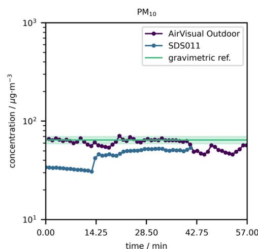
**Figure 5.**  $\text{PM}_{10}$  mass concentrations reported by the AirVisual Outdoor and SDS011 as a function of time (model aerosol 2). The green line refers to the average mass concentration over the whole measurement period according to the gravimetric reference method, while the shaded green area designates the expanded uncertainty ( $k = 2$ ; 95% confidence interval) thereof.
