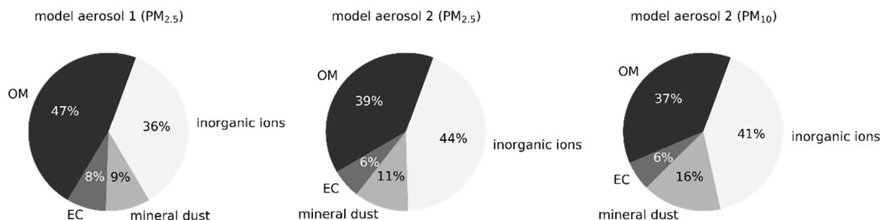
Figure 2. PM composition (%) of the two model aerosols.
