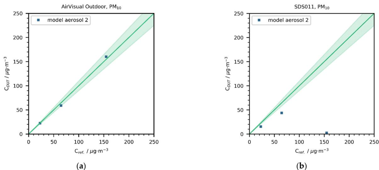
**Figure 6.** PM<sub>10</sub> mass concentrations reported by (a) the AirVisual Outdoor and (b) the SDS011 versus the gravimetric reference mass concentration. The green line denotes a perfect agreement, while the shaded green area designates a maximum 10% relative expanded uncertainty ( $k = 2$ ; 95% confidence interval) of the gravimetric reference method.
