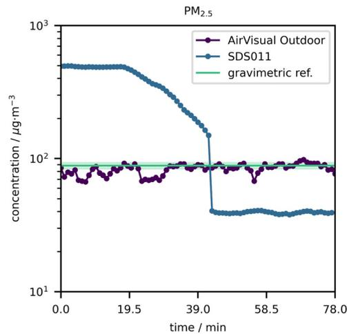
**Figure 3.**  $\text{PM}_{2.5}$  mass concentrations reported by the AirVisual Outdoor and SDS011 as a function of time for model aerosol 2. The green line refers to the average mass concentration over the whole measurement period according to the gravimetric reference method, while the shaded green area designates the expanded uncertainty ( $k = 2$ ; 95% confidence interval) thereof.
