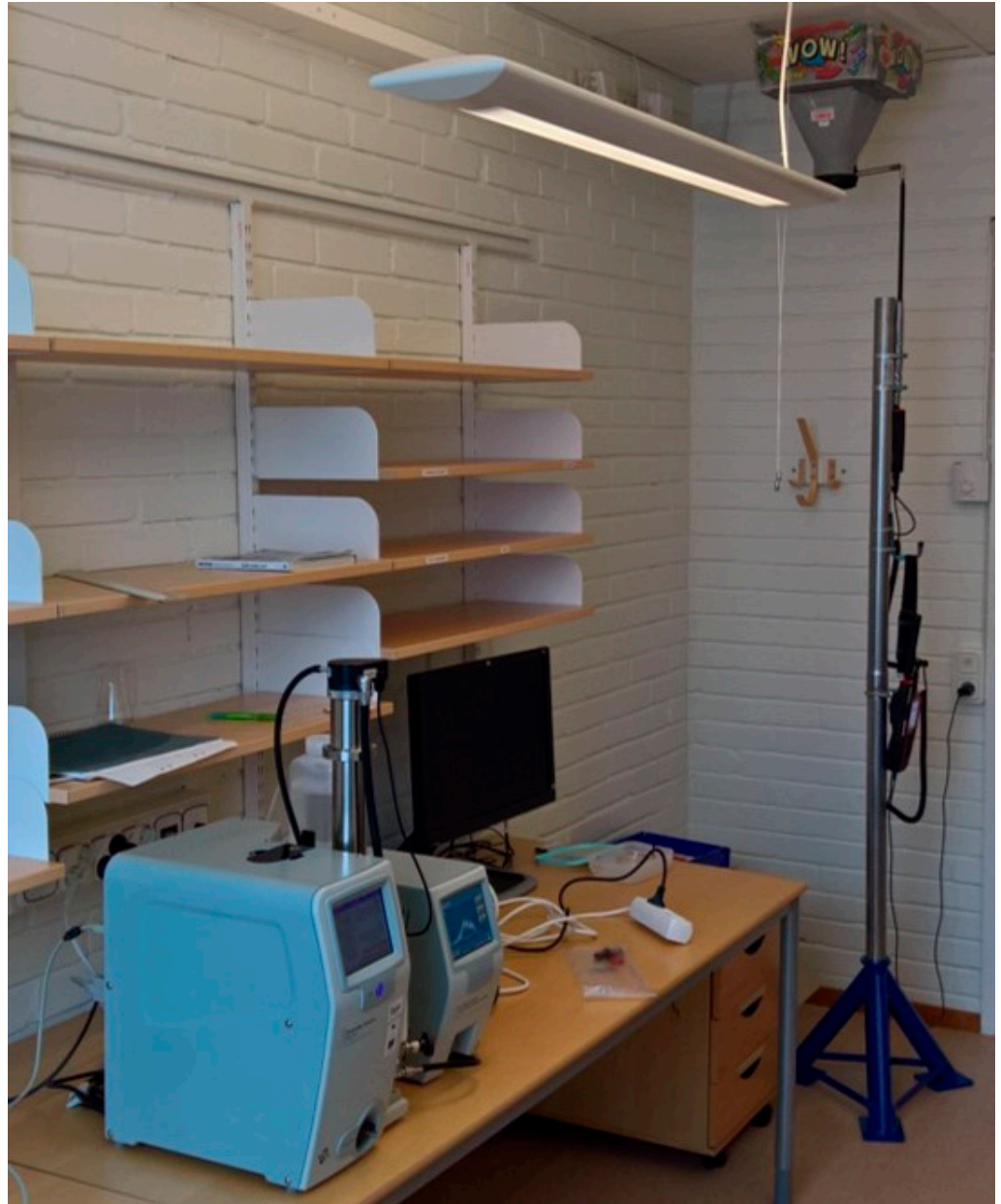
Figure 2. Measurement of nanoparticles indoors with SMPS 3938 (left) and ventilation flow with AMI310 (right).
