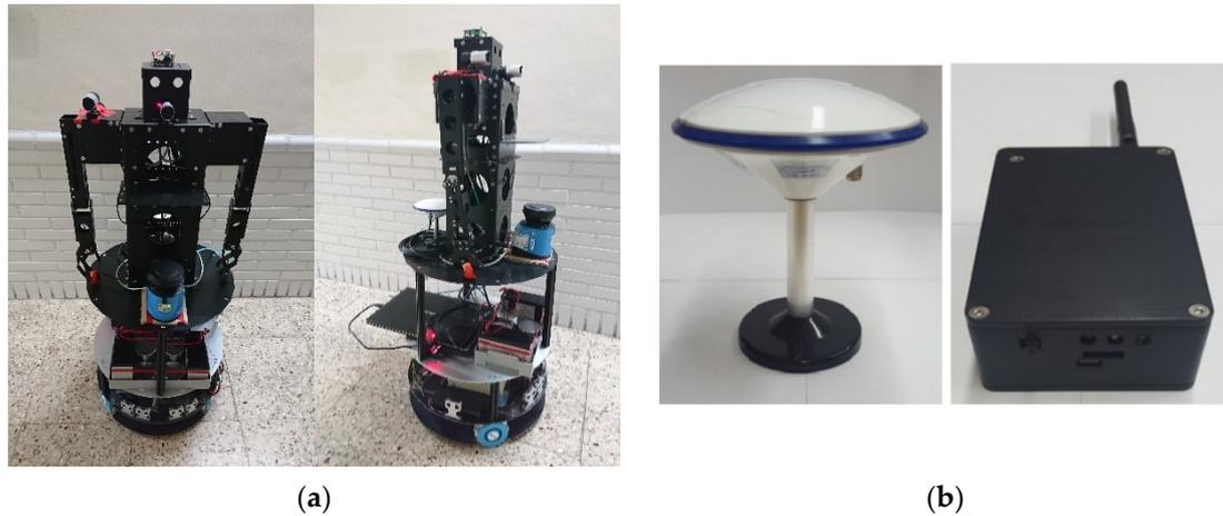
**Figure 1.** (a) The omnidirectional WMR with webcam, laser sensor, ultrasonic sensors, GNSS RTK positioning system, StarGazer positioning system, and notebook; (b) the GNSS antenna and the GNSS receiver [8].
