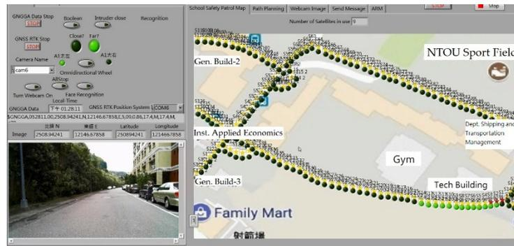
Figure 22. The robot started patrolling according to the path planning on the map.
