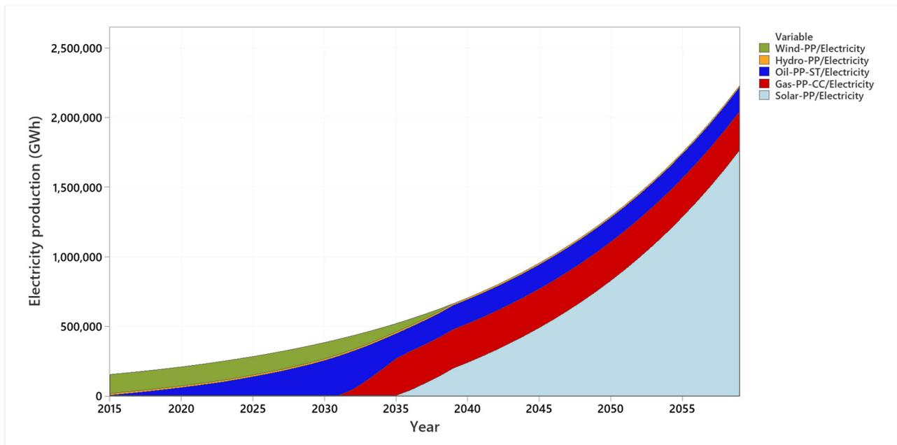
Figure 11. Balance of electricity production of all power plants for fifth scenario, solar case.
