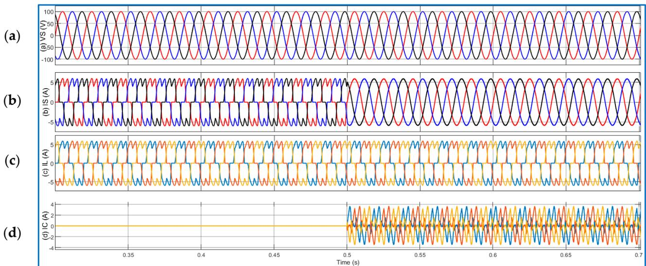
**Figure 12.** Three phase: (a) VS: supply voltage; (b) IS: supply current; (c) IL: Load current; (d) IC: compensator current.
