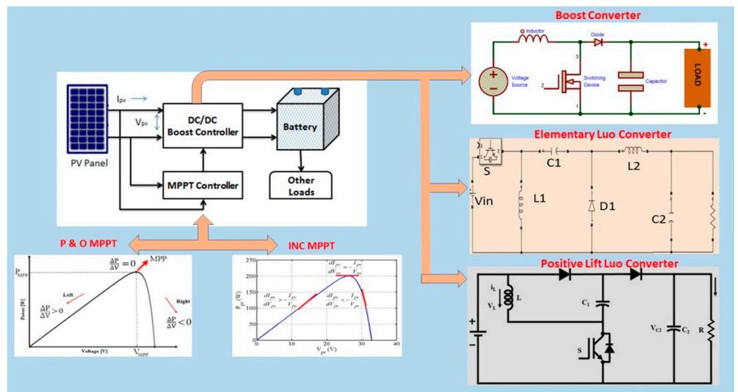
Figure 2. Different DC–DC boost converters and MPPT techniques.
