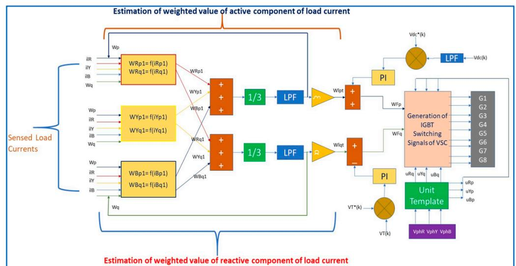
Figure 6. Block diagram of the ANN controller.
