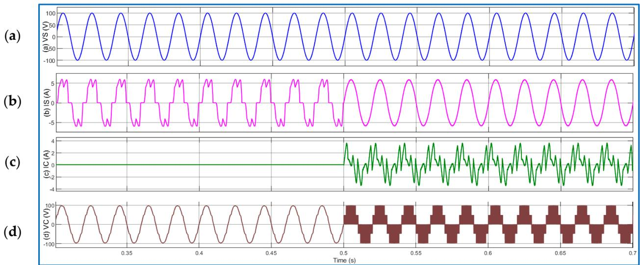
**Figure 11.** Single phase: (a) VS: supply voltage; (b) IS: supply current; (c) IC: compensator current; (d) VC: compensator voltage.
