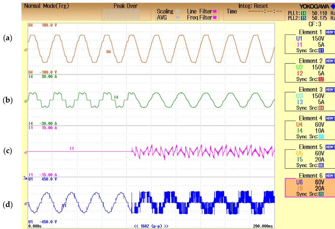
Figure 15. Single phase: (a) supply voltage; (b) supply current; (c) compensator current; (d) compensator voltage.
