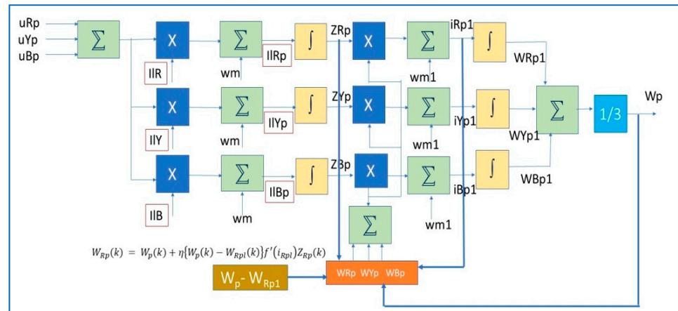
Figure 7. Configuration of backpropagation-based ANN model.
