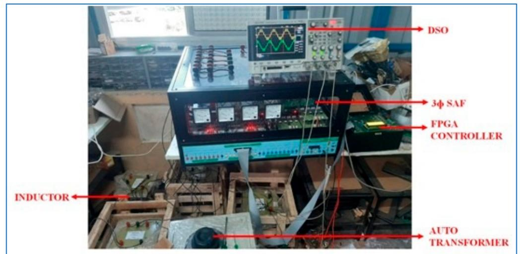
Figure 14. Experimental set-up of the DSTATCOM.
