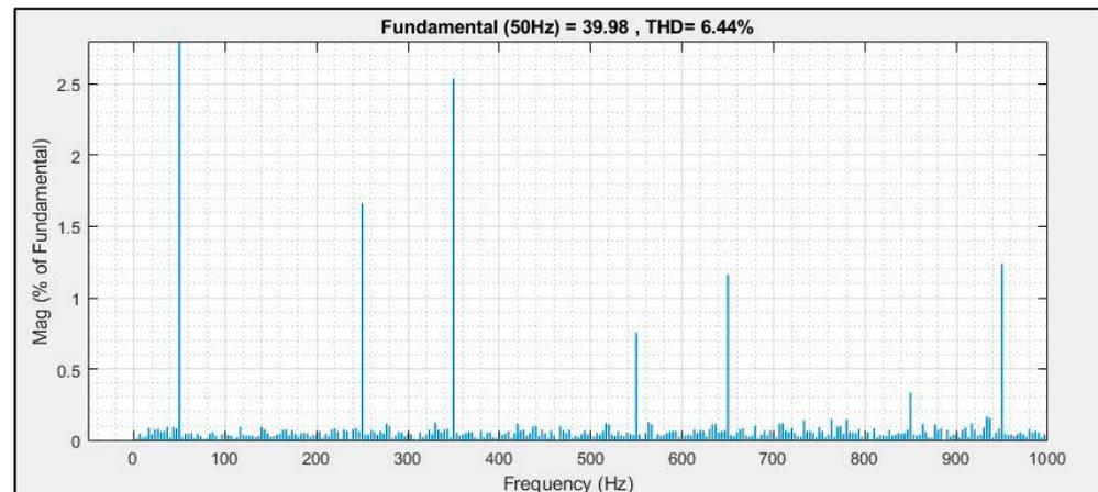
Figure 19. Source current THD using DSTATCOM with a PI Controller.
