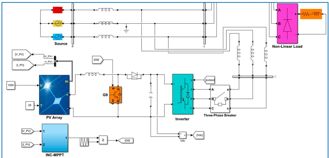
**Figure 10.** Simulink model of the grid-tied solar PV system.
