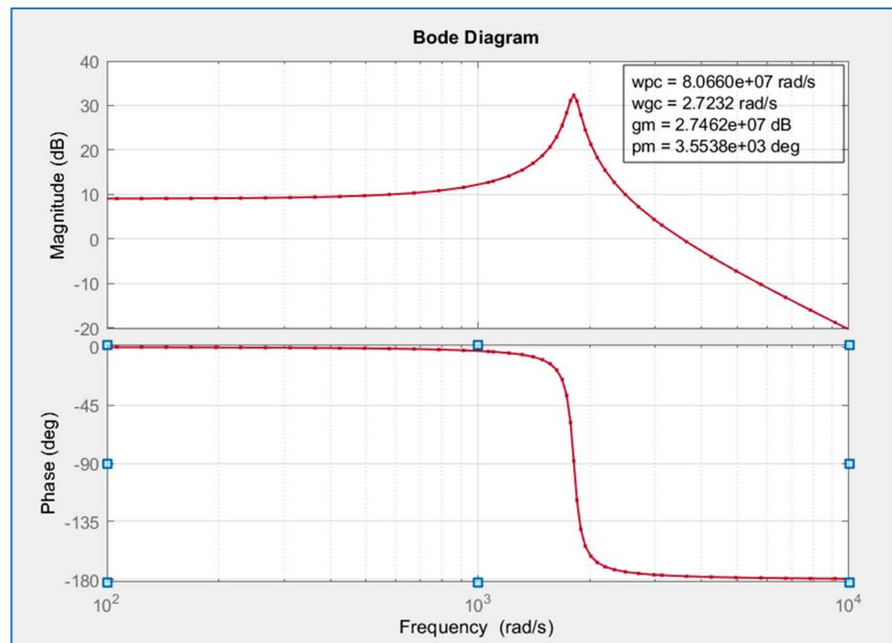
Figure 5. Bode plot of the super-lift Luo converter.
