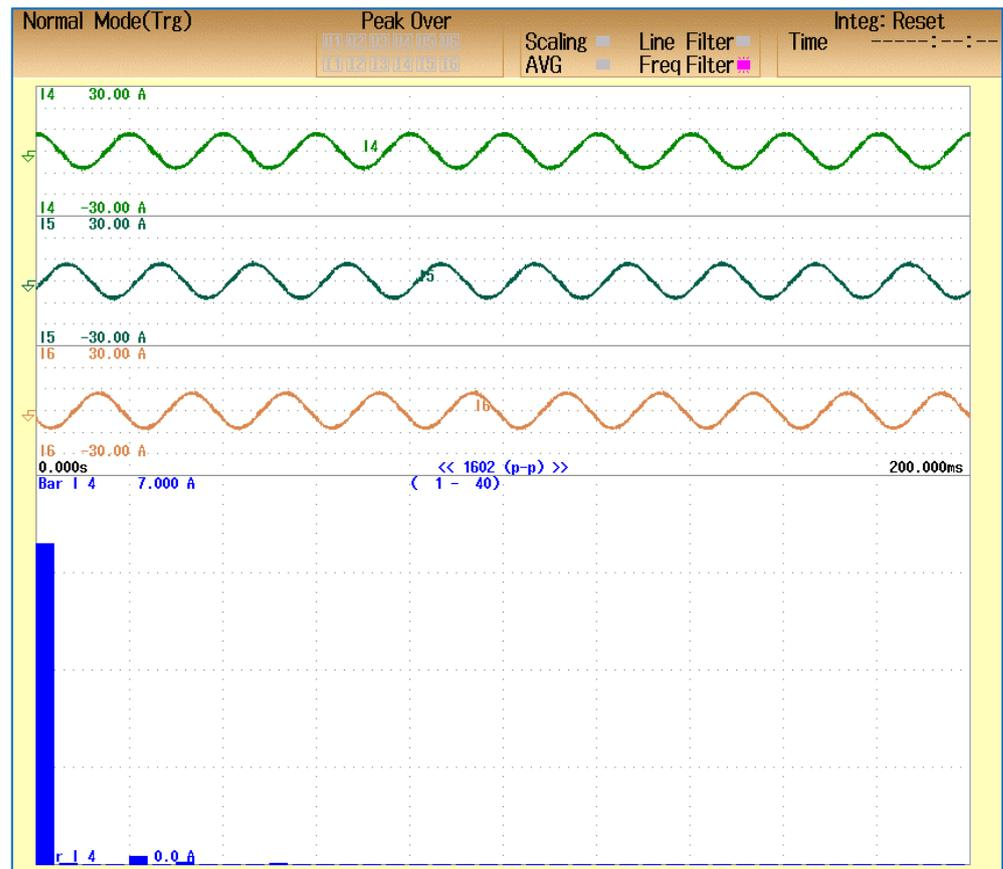
Figure 17. Supply currents of the three phases and their THD.
