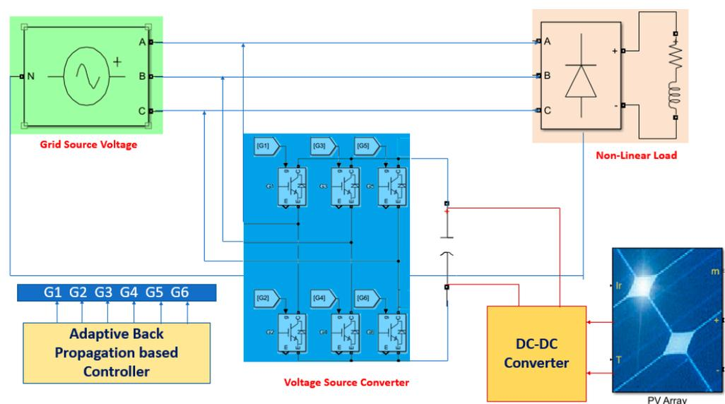
**Figure 1.** Schematic diagram of the ANN-BP control strategy for the grid-tied solar PV System.
