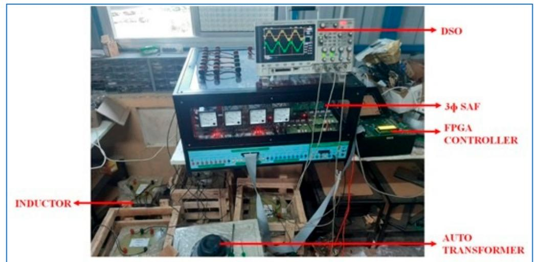
Figure 14. Experimental set-up of the DSTATCOM.
