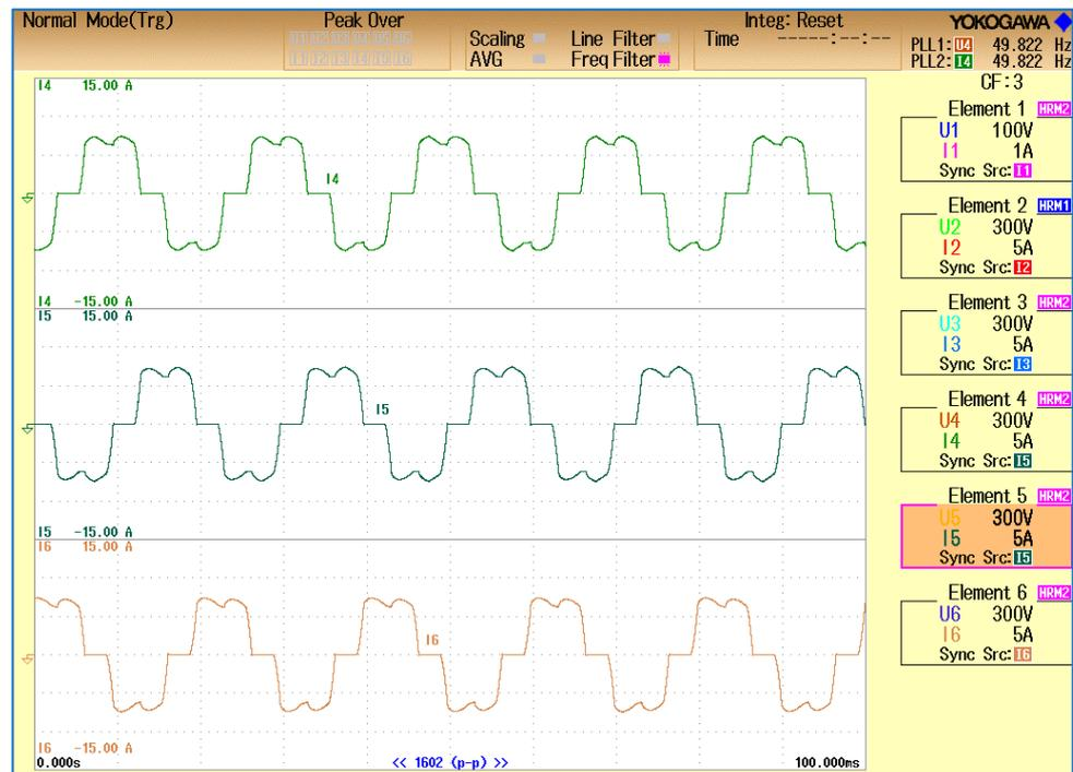
Figure 16. Load currents of the three phases.
