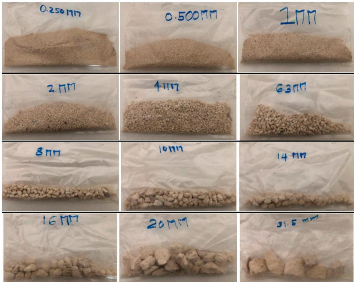
Figure 7. Digital images of TBM muck samples retained on each sieve during sieve analysis.
