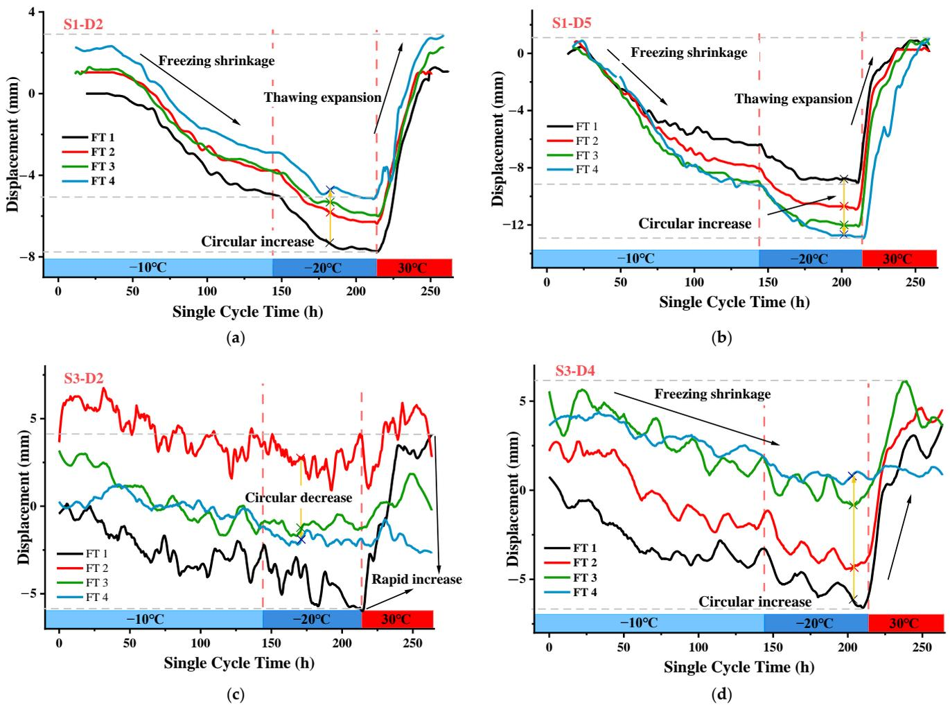
**Figure 11.** Displacement of the expansive soil slope model in four freeze-thaw cycles. (a) S1-D2; (b) S2-D5; (c) S3-D2; (d) S3-D4.
