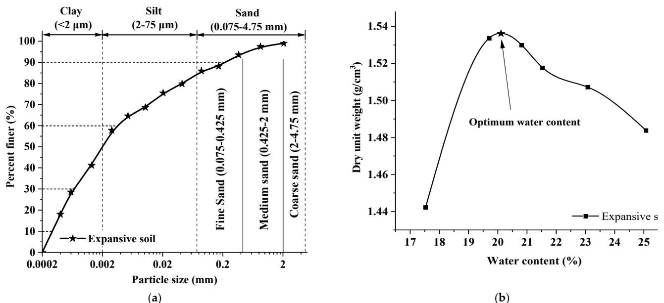
**Figure 1.** Grain-size distribution curves and compaction test for the soil. (a) Ratio and classification of different soil particles; (b) compaction curves of the soil.
