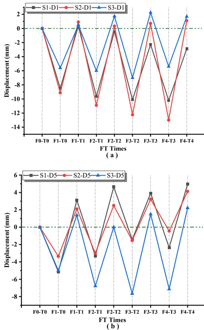
Figure 13. Slope displacement variation after freezing and thawing. (a) Slope bottom displacement; (b) slope top displacement.
