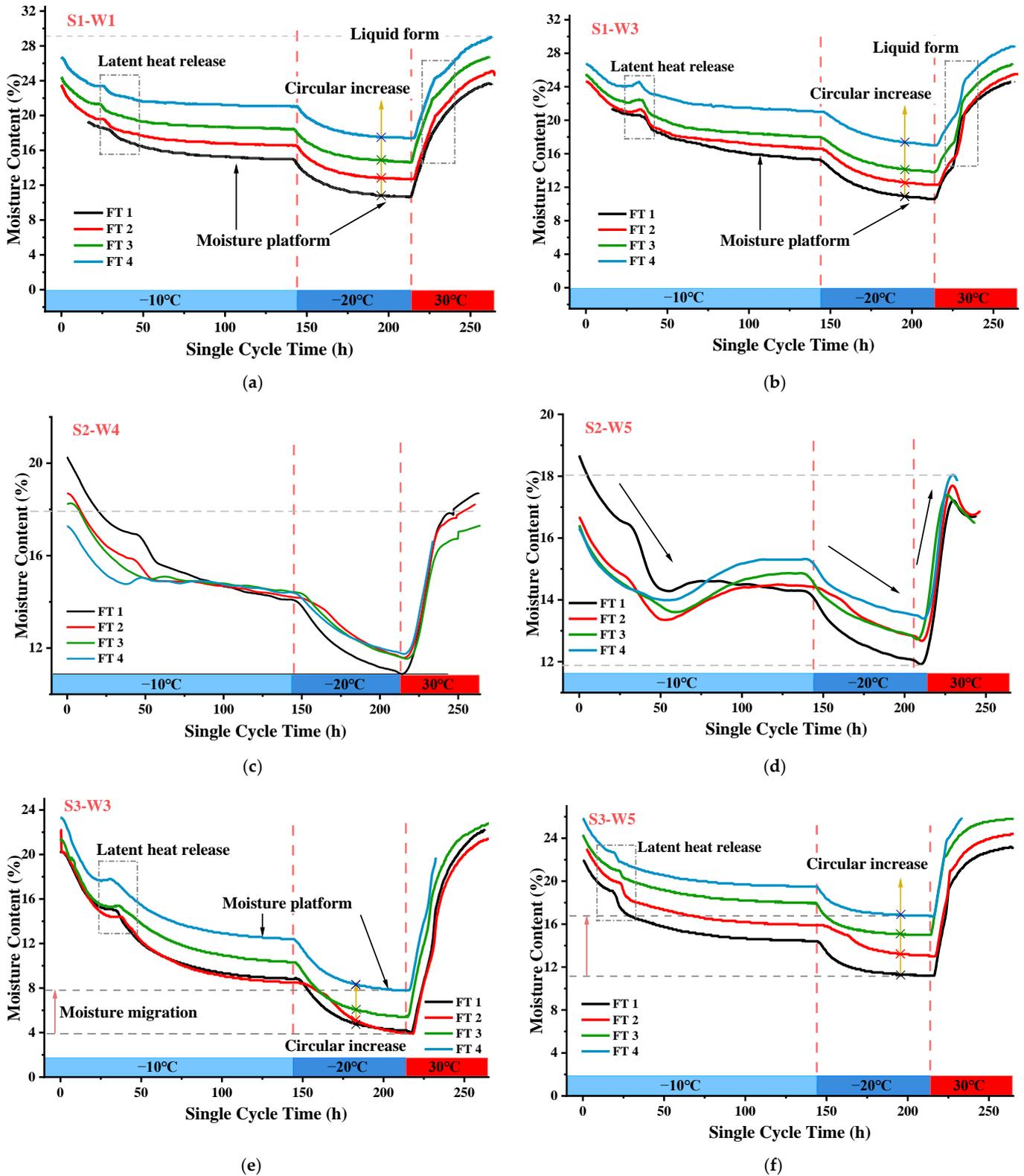
Figure 8. Moisture content of the slope model after four freeze-thaw cycles. (a) S1-W1; (b) S1-W3; (c) S2-W4; (d) S2-W5; (e) S3-W3; (f) S3-W5.
