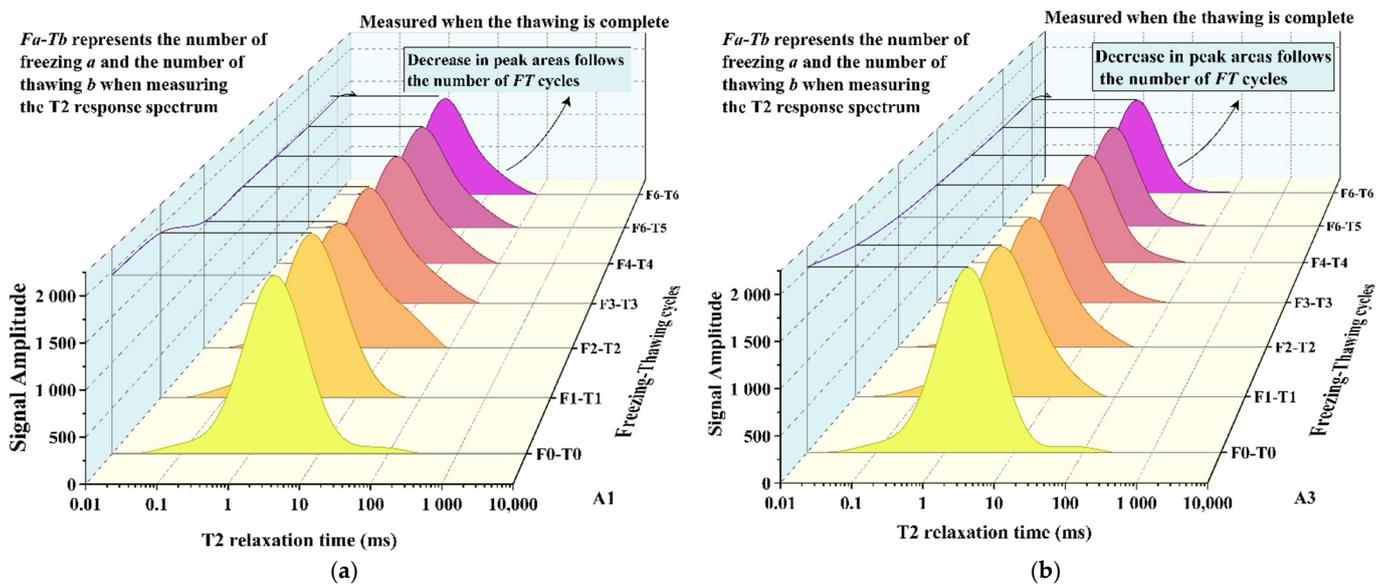
Figure 7. T<sub>2</sub> distribution of the expansive soil after six freeze-thaw cycles. (a) A1 sample test results; (b) A3 sample test results.
