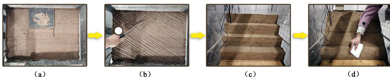
**Figure 2.** Slope preparation process. ((a) layered compaction; (b) surface scraping; (c) dismantling mold; (d) slope cutting).
