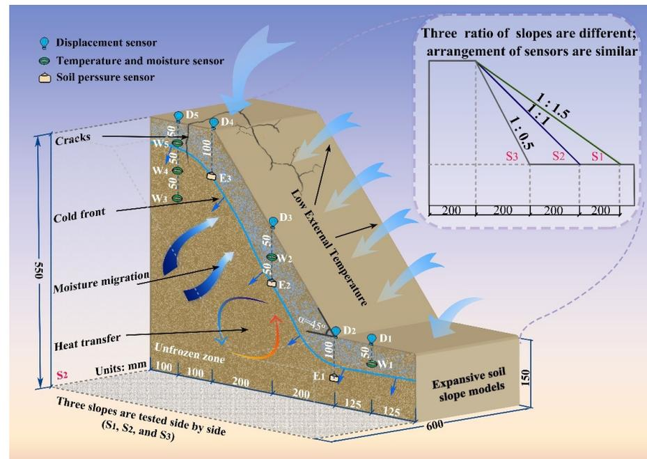
**Figure 3.** Slope freezing model and freeze-thaw monitoring system.
