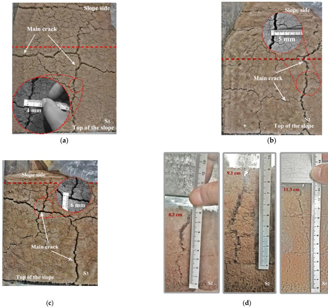
Figure 6. Crack development of the slope model after four freeze-thaw cycles (a) S<sub>1</sub> (b) S<sub>2</sub> (c) S<sub>3</sub> (d) Vertical cracks.
