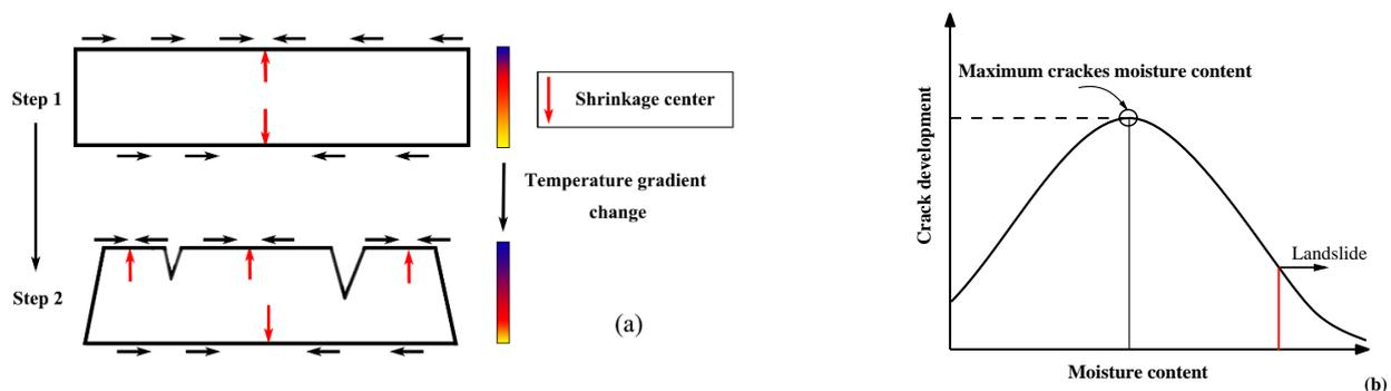
**Figure 12.** Crack development of the slope during freezing and thawing (a) formation process of freeze-thaw cracks; (b) relationship between cracks and moisture content in the freeze-thaw process.
