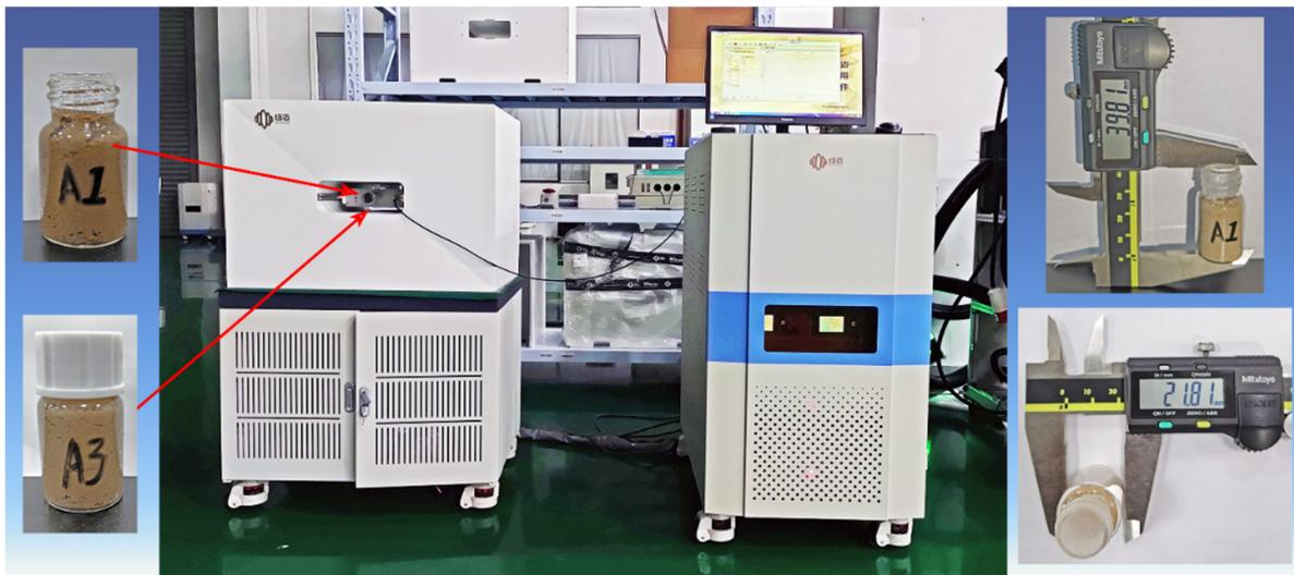
**Figure 5.** Nuclear magnetic resonance analysis instrument and test samples.
