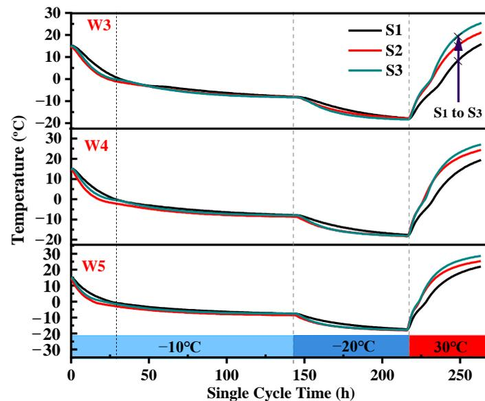
Figure 9. Temperature of slope model in one freeze-thaw cycle.
