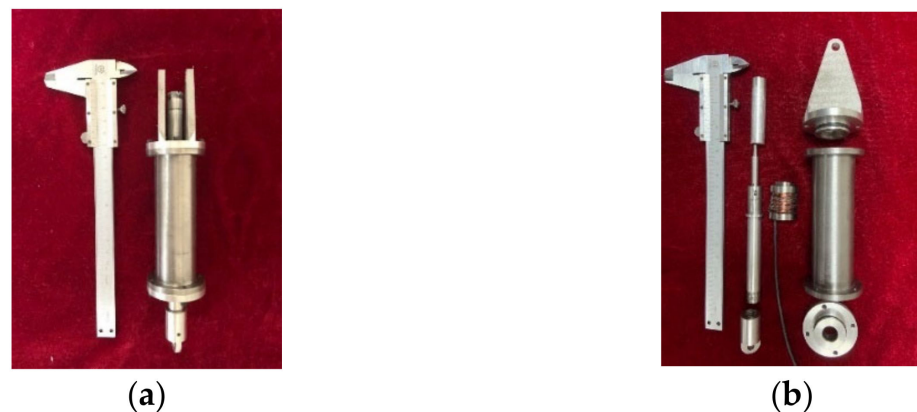
Figure 7. Prototype of the proposed MR damper. (a) Parts, (b) assembly.
