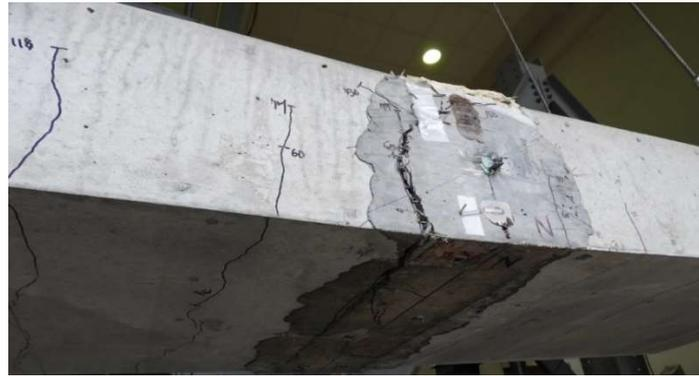
**Figure 9.** Type B specimen at end of bending test (North side).
