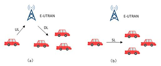
**Figure 5.** Two types of V2V connections: (a) from vehicles to vehicles with an intermediate transfer connection and; (b) directly from vehicles to other vehicles [61].
