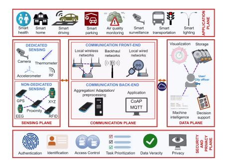
**Figure 6.** Smart city architecture defined in five planes: application (connects city and citizens), sensing (sensors measurements), communication (cloud services), data (processing and analysis) and security and privacy planes (assurance of security and privacy) [85].
