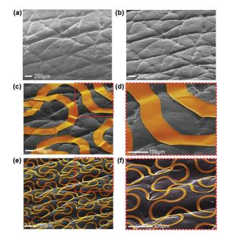
**Figure 4.** (a) Epidermal electronic system (EES) made of a skin replica created from the forearm, before and; (b) after application of a spray-on-bandage; (c) Colourized microscopy image of the EES with conductive gold films of 100  $\mu$ m and; (e) its magnified view. (d) Microscopy image of EES with gold films of 10  $\mu$ m and; (f) its magnified view [48].
